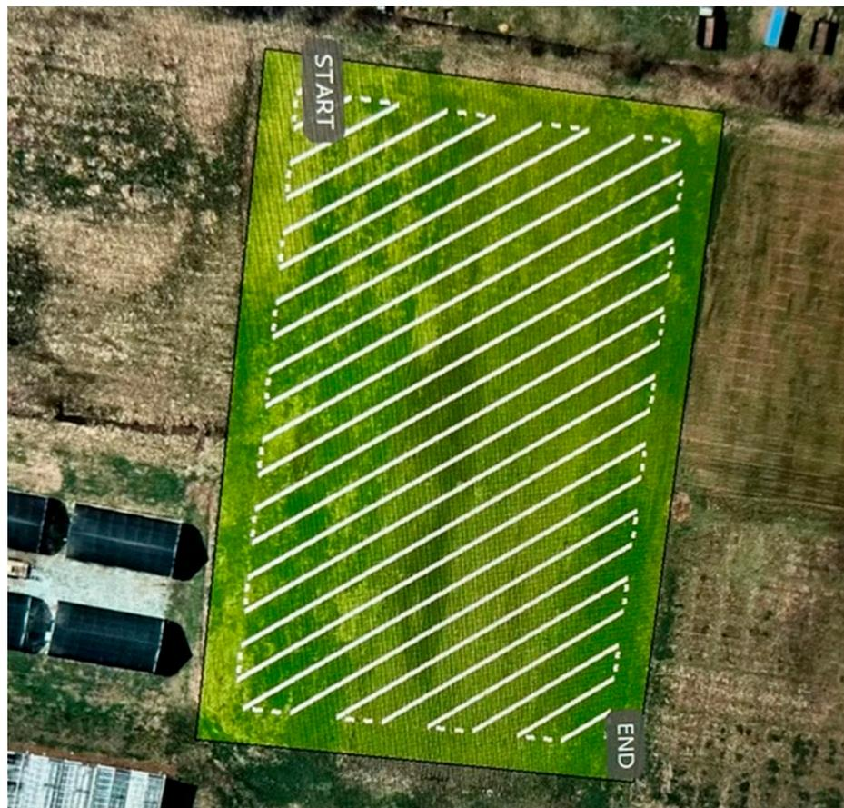
**Figure 4.** The drone path for the acquisition of field sampling pictures.
