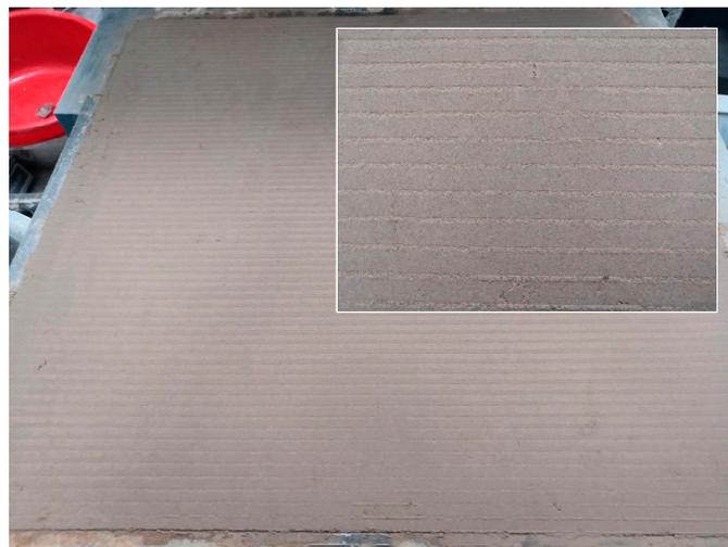
**Figure 7.** Shear interface after the test was completed.
