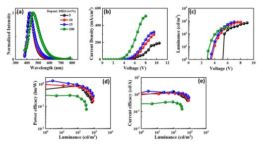
**Figure 13.** The electroluminescent (EL) properties of the device with emitter DB24 doped in CBP host matrix at varying concentrations showing (**a**) EL spectra, (**b**) current density–voltage, (**c**) luminance–voltage, (**d**) power efficacy–luminance, and (**e**) current efficacy–luminance characteristics.
