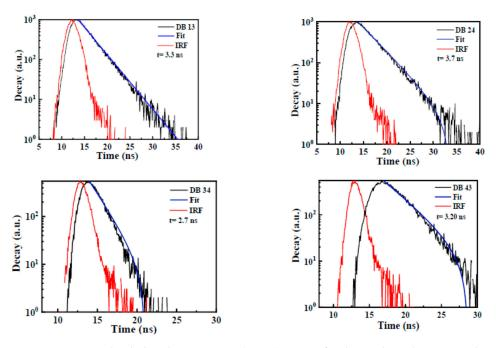
**Figure 7.** Time-resolved photoluminescence (TRPL) spectra for the PL decay kinetics analysis of the compounds DB 13, DB 24, DB 34, and DB 43.
