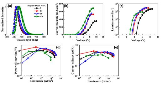
**Figure 12.** The electroluminescent (EL) properties of the device with emitter DB13 doped in CBP host matrix at varying concentrations showing (**a**) EL spectra, (**b**) current density–voltage, (**c**) luminance–voltage, (**d**) power efficacy–luminance, and (**e**) current efficacy–luminance characteristics.
