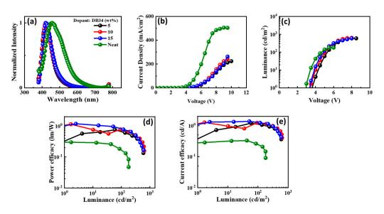
**Figure 14.** The electroluminescent (EL) properties of the device with emitter DB34 doped in CBP host matrix at varying concentrations showing (**a**) EL spectra, (**b**) current density–voltage, (**c**) luminance–voltage, (**d**) power efficacy–luminance, and (**e**) current efficacy–luminance characteristics.
