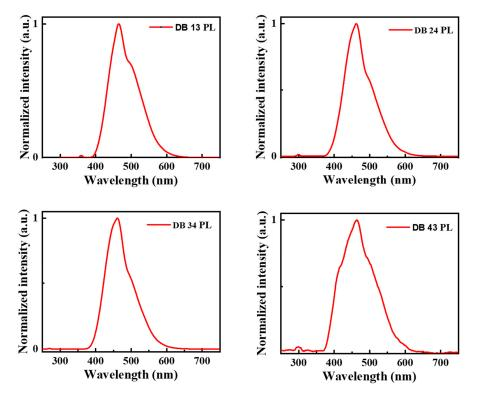
Figure 5. Photoluminescence (PL) spectra of the compounds DB13, DB24, DB34, and DB43.
