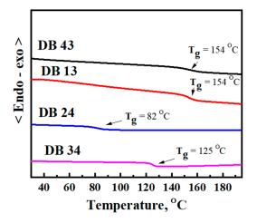
**Figure 10.** DSC curves of second heating for estimating glass transition temperatures ( $T_g$ ) of the compounds DB13, DB24, DB34, and DB43.
