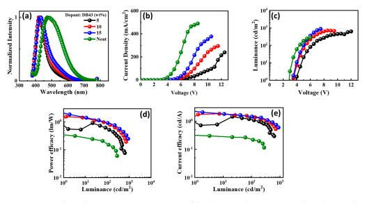
**Figure 15.** The electroluminescent (EL) properties of the device with emitter DB43 doped in CBP host matrix at varying concentrations showing (**a**) EL spectra, (**b**) current density–voltage, (**c**) luminance–voltage, (**d**) power efficacy–luminance, and (**e**) current efficacy–luminance characteristics.
