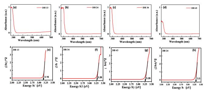
**Figure 4.** (**a**–**d**) Ultraviolet–visible absorbance (UV abs) spectra and (**e**–**h**) Tauc plot, represent the absorption wavelength and bandgap, respectively, of the compounds DB13, DB24, DB34 and DB43.
