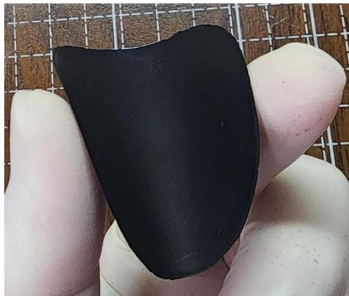
**Figure 1.** Photo of BP after the vacuum filtration process. BP is ductile, and MWCNTs are evenly distributed.
