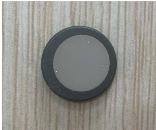
Figure 1. Sintered aluminum electrode sample.
