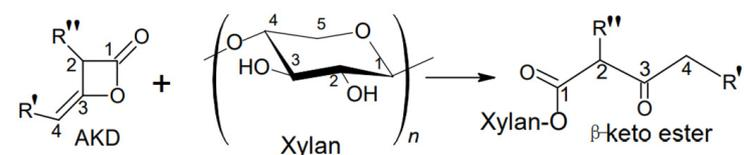
**Figure 1.** Reaction of xylan hemicellulose with AKD. Note that  $R'$  and  $R''$  are typically in the range of C4–C16 ( $C_{14}H_{29}$ ).
