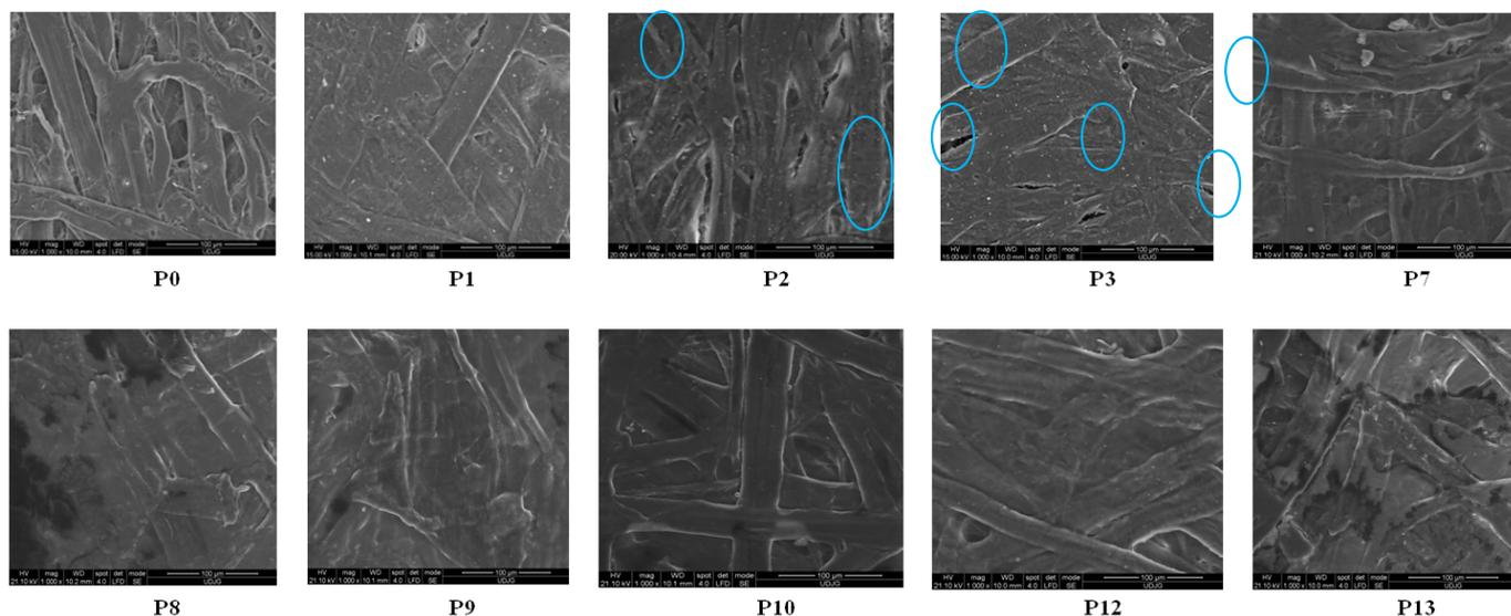
**Figure 5.** SEM images of paper samples coated in single and two successive layers based on xylan derivatives and chitosan. P0: base paper. Homogeneous coatings in single layer—P1: 100Xy; P2: 100XyAKD; P3: 100XyAc; P7: 50Xy50Ch; P8: 50XyAKD50Ch; P9: 50XyAc50Ch; P10: 100Ch. Composite coatings in two layers—P12: 100XyAKD + 100Ch; P13: 100XyAc + 100Ch. The blue circles highlight the non-uniformities and cracks in the coating layer structure.
