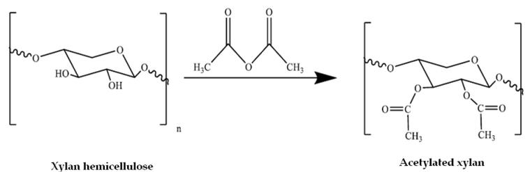
**Figure 2.** Reaction of xylan with acetic anhydride.
