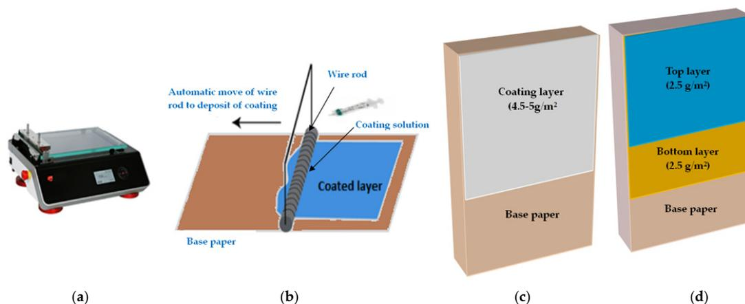
**Figure 3.** Representation of laboratory coating papers: (a) automatic coating applicator; (b) details of the coating deposition on the paper surface; (c) homogeneous coating in single layer; (d) composite coatings in two successive layers.
