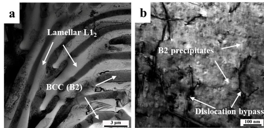
**Figure 5.** TEM images of 650-alloy: (a) low magnification and (b) dislocation morphology around  $B_2$  phase.
