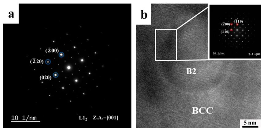
Figure 3. TEM images of  $\text{Al}_{1.1}\text{CoCrFeNi}_{2.1}$ : (a) SAED corresponding to the  $L_{12}$ ; (b) HRTEM image of BCC ( $B_2$ ).
