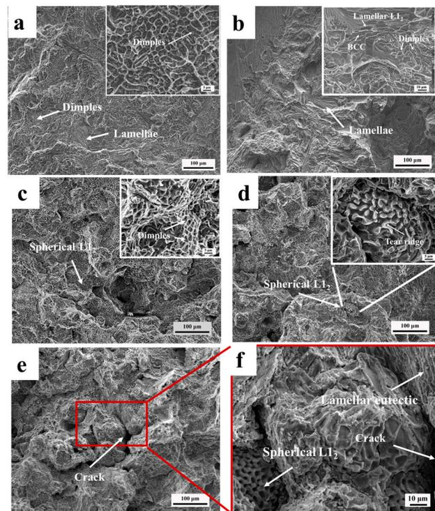
**Figure 9.** Fracture morphologies of (a)  $-100$ -alloy; (b) RT-alloy; (c) 650-alloy; (d) 750-alloy; (e) 850-alloy; (f) magnified spherical  $\text{L}_{12}$  and lamellar eutectic of 850-alloy.
