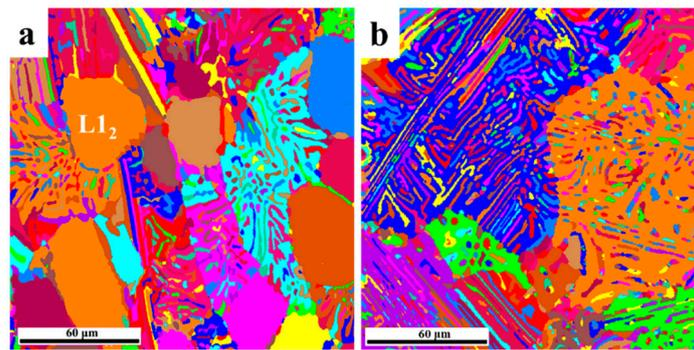
**Figure 6.** EBSD grain distribution maps of (a) –100-alloy; (b) RT-alloy.
