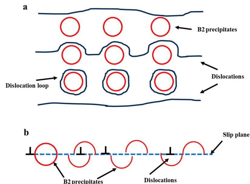
**Figure 10.** Schematic illustration of (a) Orowan bypass mechanism and (b) dislocation cutting mechanism.
