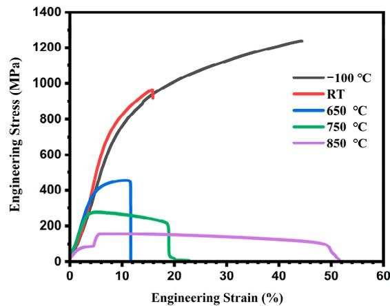
**Figure 8.** Mechanical properties of hypereutectic  $\text{Al}_{1.1}\text{CoCrFeNi}_{2.1}$  alloy at different temperatures.
