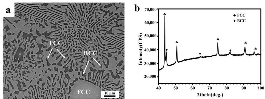
Figure 1. (a) SEM image and (b) XRD pattern of hypereutectic  $\text{Al}_{1.1}\text{CoCrFeNi}_{2.1}$ .
