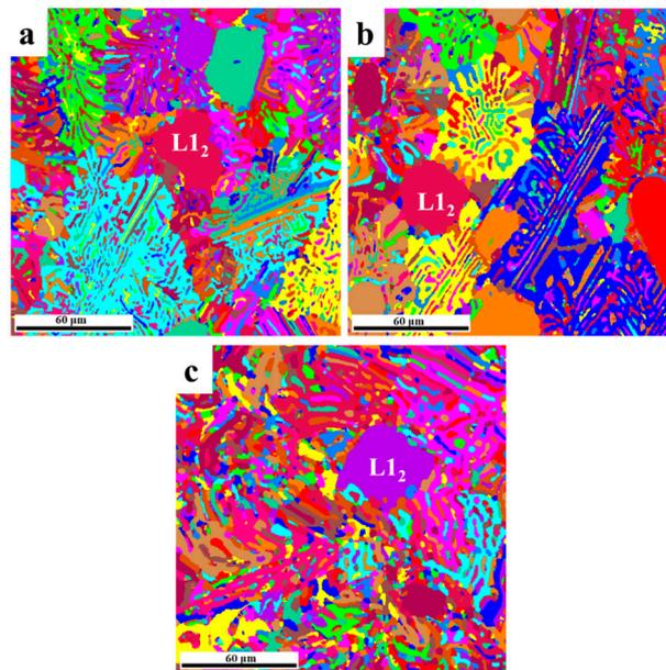
**Figure 7.** EBSD grain distribution maps of (a) 650-alloy; (b) 750-alloy; (c) 850-alloy.
