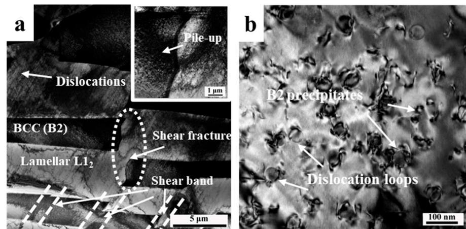
**Figure 4.** TEM images of RT-alloy: (a) low magnification and (b) dislocation morphology around  $B_2$  phase.
