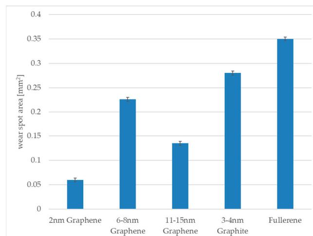
**Figure 8.** Wear spot areas of steel balls measured under 3D laser scanning microscope tested against dry lubricants under 660 MPa contact pressure after sliding test.
