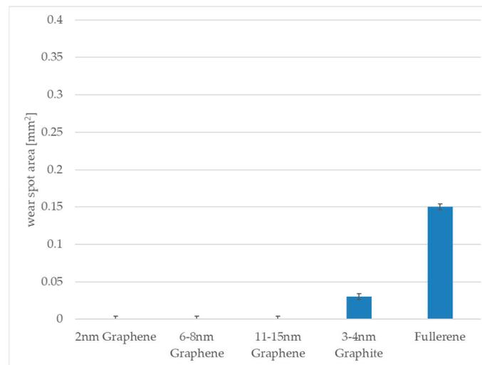
**Figure 9.** Wear spot areas of steel balls measured under 3D laser scanning microscope tested against pre-rolled dry lubricants under 660 MPa contact pressure after sliding test.
