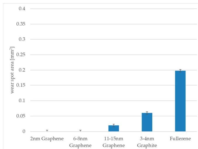
**Figure 10.** Wear spot areas of steel balls measured under 3D laser scanning microscope tested against pre-rolled dry lubricants under 830 MPa contact pressure after sliding test.
