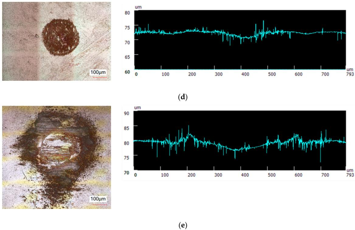
**Figure 11.** Wear spot of steel balls under 3D laser scanning microscope tested against pre-rolled dry lubricants under 830 MPa contact pressure after sliding test for (a) 2 nm thick graphene platelets, (b) 6–8 nm thick graphene platelets, (c) 11–15 nm thick graphene platelets, (d) 3–4 nm nano-graphite, and (e) fullerene.
