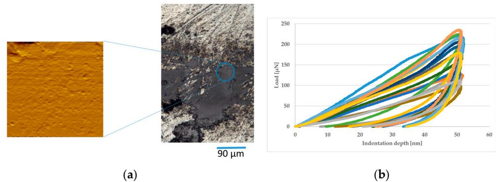
**Figure 14.** Nanoindentation study on pre-rolled 6–8 nm thick graphene platelets under 660 MPa: (a) surface for nanoindentational study after test (on the left: scanning probe microscopy of the surface  $25 \times 25 \mu\text{m}$ ; on the right: light microscopic view) and (b) nanoindenters on surface after test with pre-rolled 6–8 nm thick graphene platelets under 660 MPa.
