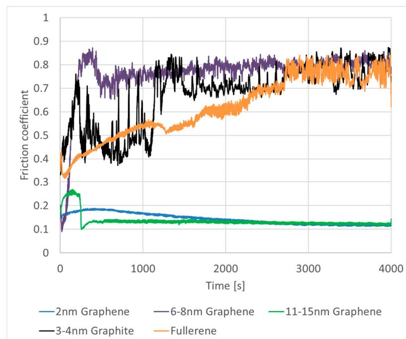
**Figure 5.** Friction coefficient on steel coated with graphene platelets, nano-graphite, and fullerene without pre-rolling, tested under 660 MPa.
