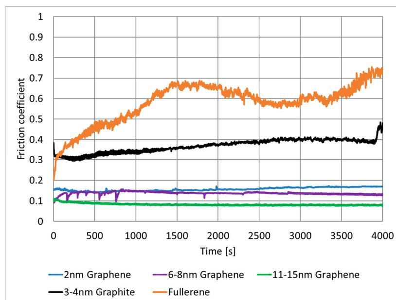
**Figure 6.** Friction coefficient on steel coated with graphene platelets, nano-graphite, and fullerene with pre-rolling, tested under 660 MPa.
