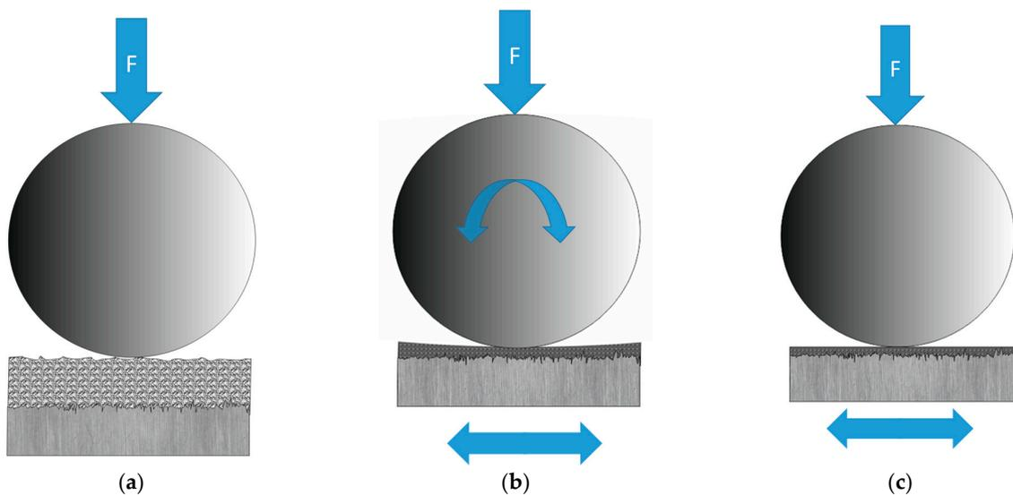
**Figure 3.** Test principle: (a) loading the dry-coated sample, (b) pre-rolling under load and subsequent compacting with movable mounted ball, (c) sliding test with fixed ball on compacted dry lubricant coating.
