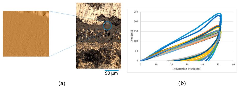
**Figure 15.** Nanoindentation surface study on pre-rolled 6–8 nm thick graphene platelets under 830 MPa: (a) surface for nanoindentational study after test (on the left: scanning probe microscopy of the surface  $25 \times 25 \mu\text{m}$ ; on the right: light microscopic view) and (b) nanoindenters on surface after test with pre-rolled 6–8 nm thick graphene platelets under 830 MPa.
