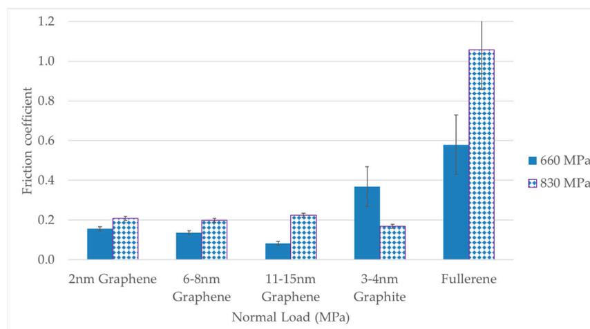
**Figure 17.** Comparison of frictional coefficients for pre-rolled dry lubricants under 660 MPa and 830 MPa pressure, after pre-rolling.
