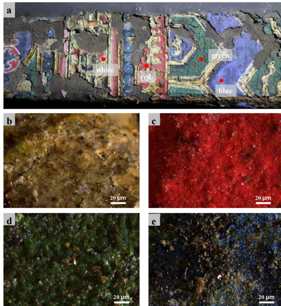
**Figure 2.** (a) Four pigment samples collected from the color painting on the beam: (b) white, (c) red, (d) green, and (e) blue pigments, as labeled with red dots. All samples were observed under 20× magnifications.
