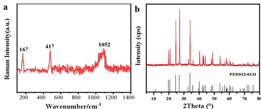
**Figure 3.** Raman spectra (a) and X-ray diffraction spectra (b) of the white pigments (The black line is a standard PDF card, obtained from the Jade software, and the red line is the test result).
