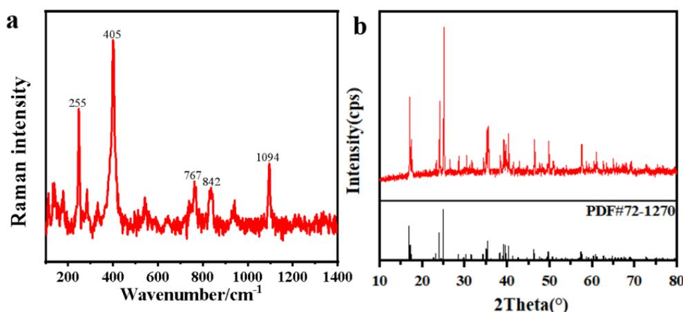
**Figure 6.** (a) Raman spectra of blue pigments; (b) X-ray diffraction spectra of blue pigments (The black line is a standard PDF card, obtained from the Jade software, and the red line is the test result).
