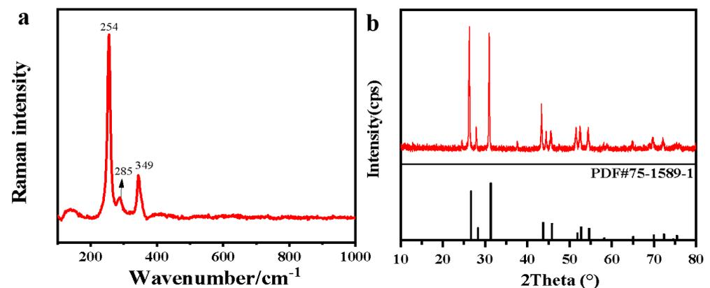
**Figure 4.** (a) Raman spectra for red pigments; (b) X-ray diffraction spectra of red pigments.
