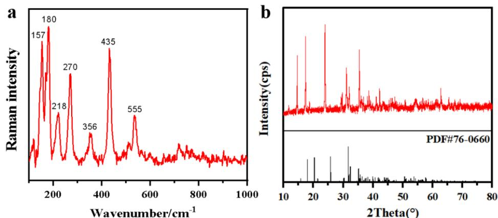
**Figure 5.** (a) Raman spectra of green pigments; (b) X-ray diffraction spectra of green pigments (The black line is a standard PDF card, obtained from the Jade software, and the red line is the test result).
