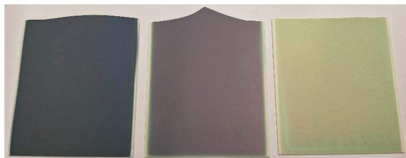
**Figure 4.** Visual appearance of 2  $\mu\text{m}$  thick  $\text{WO}_x$  films on  $\text{Al}_2\text{O}_3$  ceramic substrates, deposited at different setpoint values for controlling the inlet flow of  $\text{O}_2$  into the vacuum chamber. From left to right: 70% ( $\text{WO}_{x_1}$ ), 90% ( $\text{WO}_{x_2}$ ), and 130% ( $\text{WO}_{x_3}$ ).
