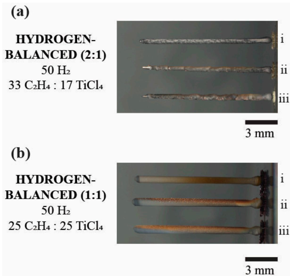
**Figure 8.** The digital image comparing the two hydrogen-balanced mixtures. (a) The hydrogen-balanced (2:1) deposit of three fibers. (b) The hydrogen-balanced (1:1) deposit of three fibers. Note the bronze color for the (1:1) condition vs. the (2:1) condition. The numerals i, ii, and iii denote the sequence of the fiber growth.
