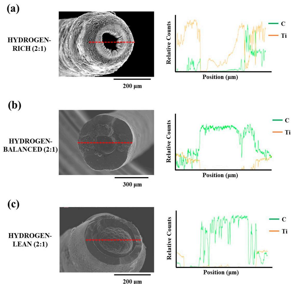
**Figure 5.** Line profiles (shown by the red line) with corresponding XEDS data for the (a) Hydrogen-rich (2:1) (b) Hydrogen-balanced (2:1) and (c) Hydrogen-lean (2:1) deposits.
