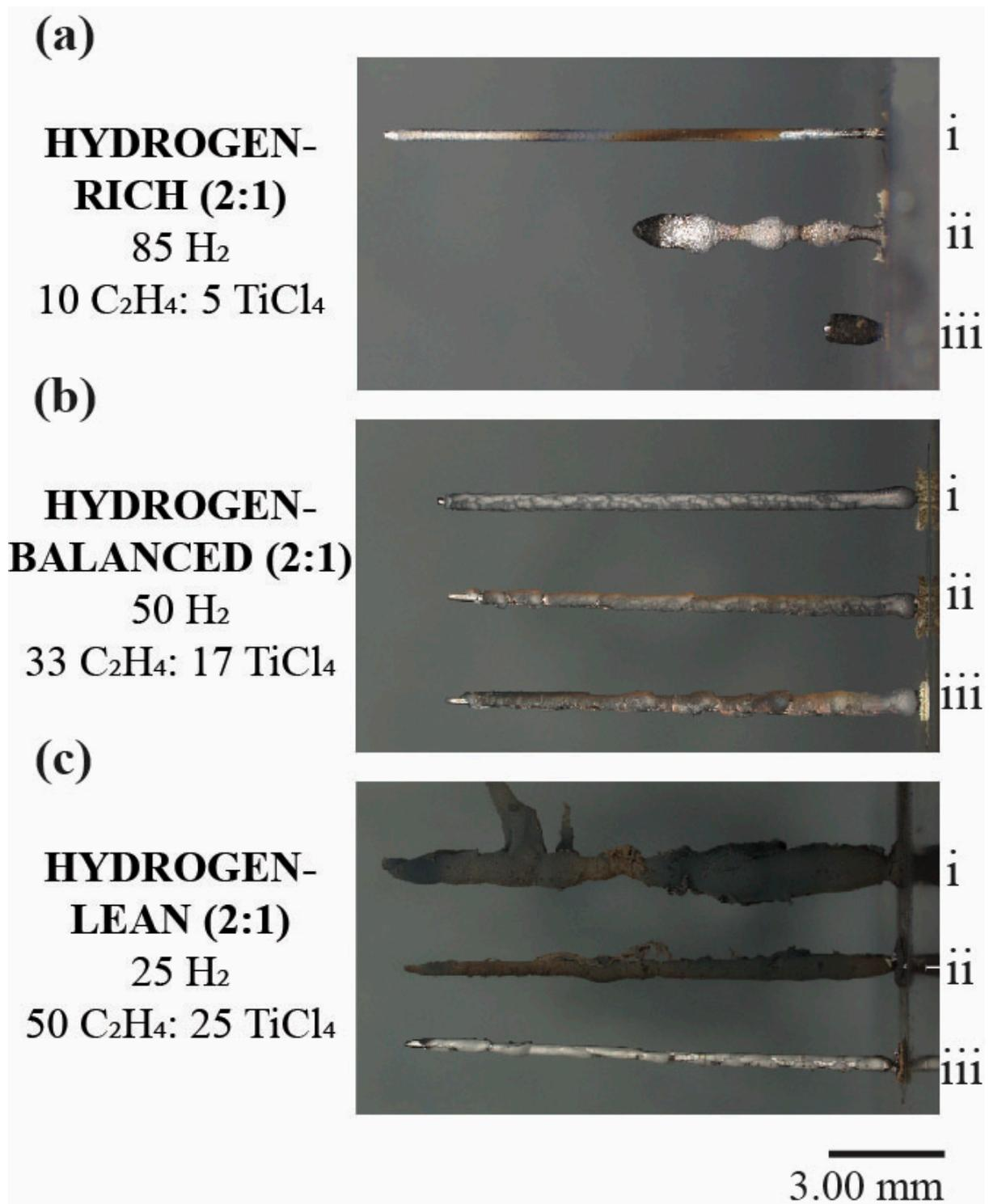
**Figure 3.** Digital images of TiC fibers in the sequence of their subsequential growth sequence of i, ii, and iii, for the first, second, and third deposition for the (a) Hydrogen-rich (b) Hydrogen-balanced and (c) Hydrogen-lean conditions. The numerals i, ii, and iii denote the sequence of the fiber growth with i being the first, ii being the second, and iii being the third.
