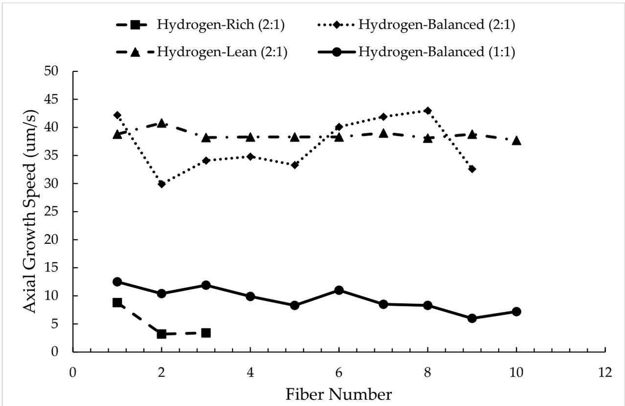
Figure 6. Growth rate as the number of sequential fibers for various precursor mixtures.
