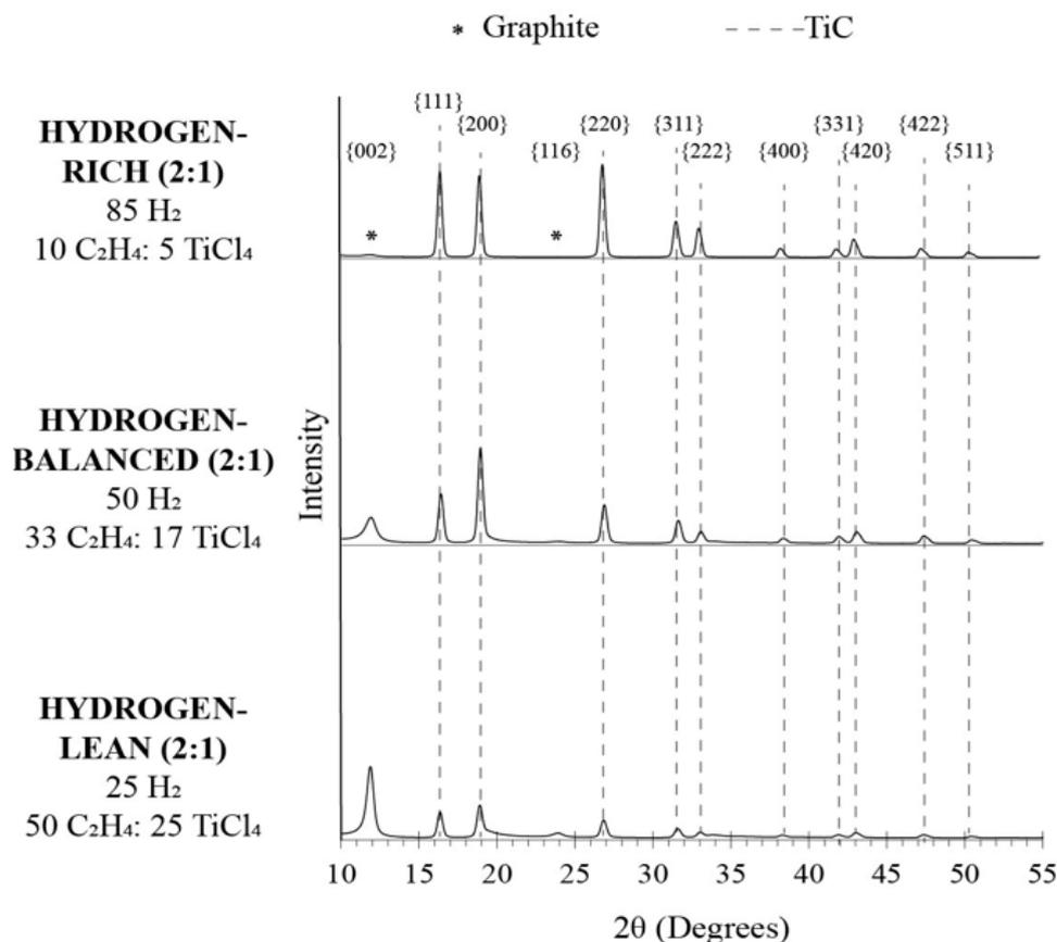
**Figure 4.** XRD data showing peaks correlating to graphite and TiC peaks.
