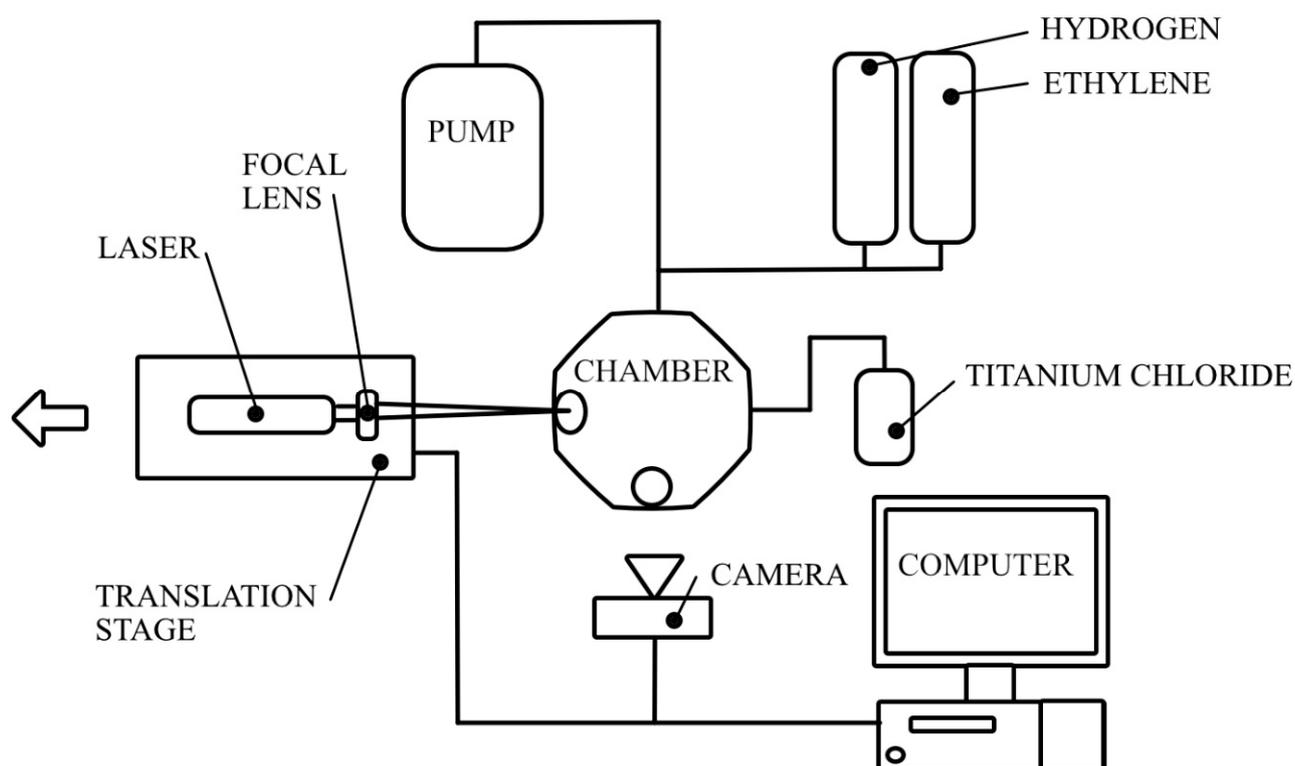
**Figure 1.** A schematic of the LCVD setup.
