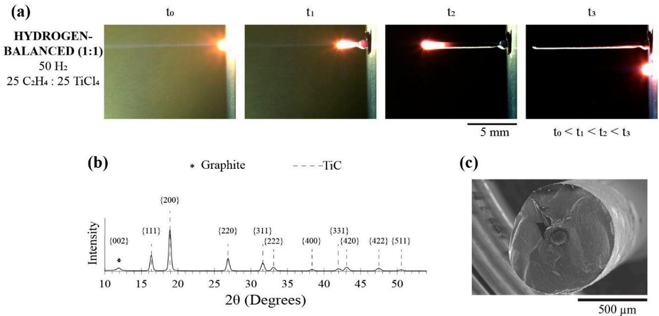
Figure 7. (a) Time-lapse images of the growth progression, (b) XRD and (c) SEM image of the hydrogen-balanced (1:1) condition fiber.
