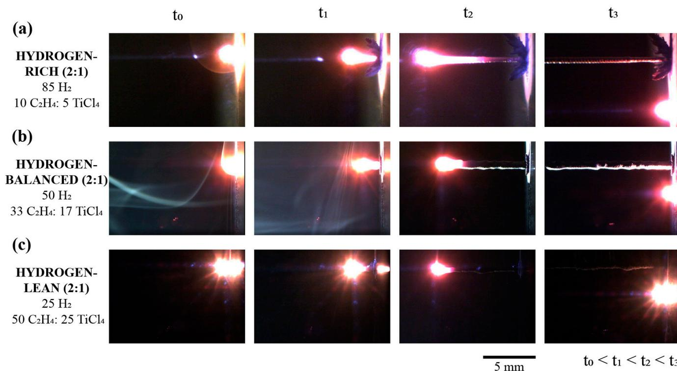
**Figure 2.** Series of time-lapse images for the 2 C<sub>2</sub>H<sub>4</sub>:1 TiCl<sub>4</sub> mixtures with hydrogen for the TiC fiber growth. (a) Hydrogen-rich (b) Hydrogen-balance and (c) Hydrogen-lean mixtures.
