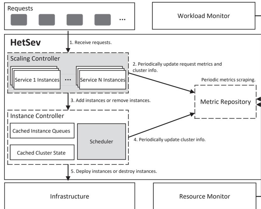
**Figure 4.** HetSev architecture. The boxes with dashed borders are the three main components of HetSev. The gray boxes are the controller-specific components which were re-implemented in our approach and deployed within a cluster manager (e.g., Kubernetes). The numbered arrows correspond to the typical workflow of HetSev.
