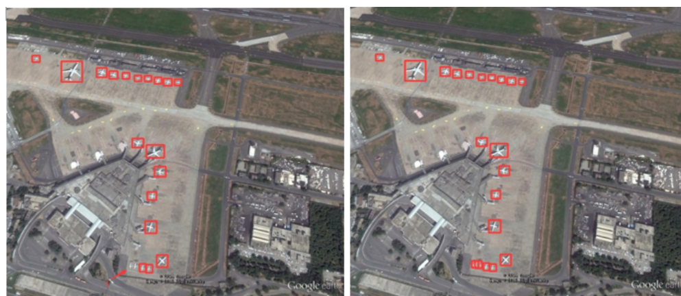
Figure 12. Multi-scale small target missed detections in complex environments. The (left) side displays the identification outcomes of YOLOv5s, while the (right) side exhibits the outcomes of YOLO-GCRS.
