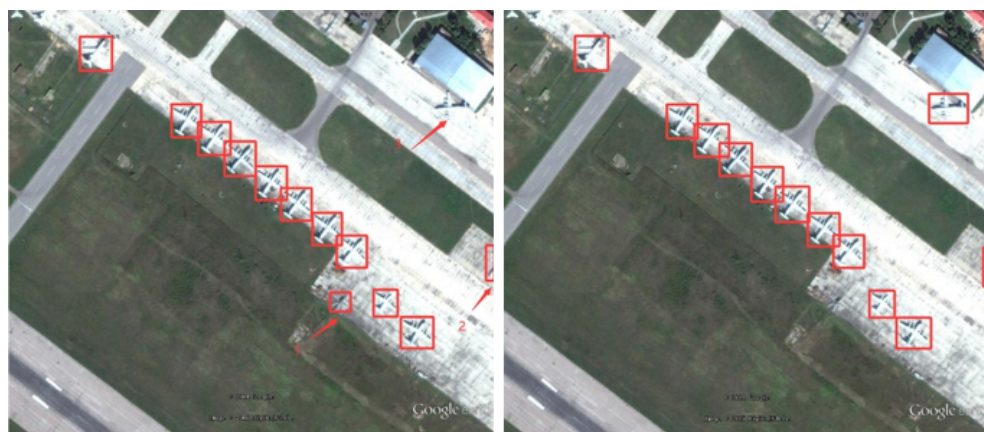
Figure 11. Missed and false detections of small targets in complex backgrounds. The (left) side displays the identification outcomes of YOLOv5s, while the (right) side exhibits the outcomes of YOLO-GCRS.
