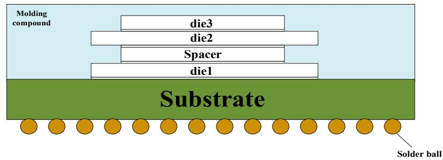
Figure 17. Schematic diagram of a three-layer cantilever and pyramid combination package.
