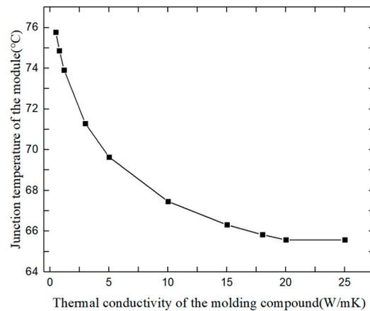
**Figure 3.** Junction temperature versus thermal conductivity of the molding compound.
