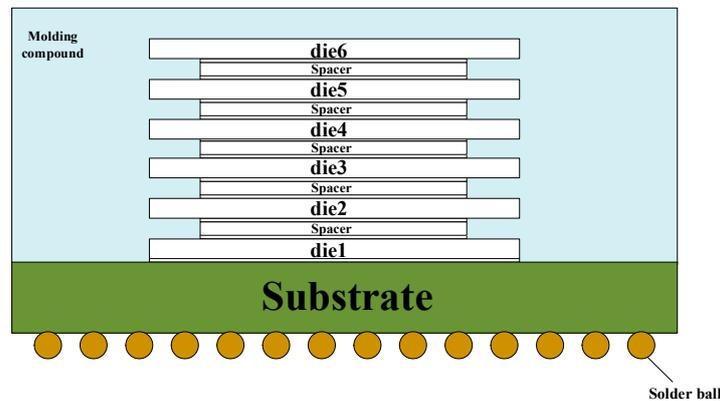
Figure 10. Schematic diagram of a six-layer cantilever stacked package.
