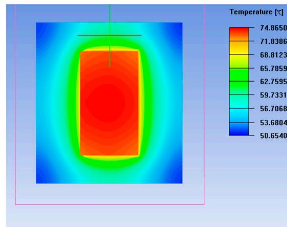
**Figure 2.** The initial temperature distribution of the stagger-stacked DDR module.
