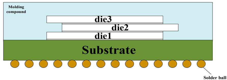
Figure 18. Schematic diagram of a three-layer stagger-stacked DDR module.
