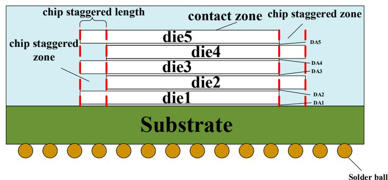
Figure 1. The whole structure of the stagger-stacked DDR module.
