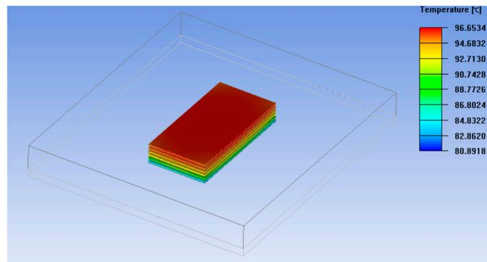
Figure 12. Initial temperature distribution of six-layer cantilever package.
