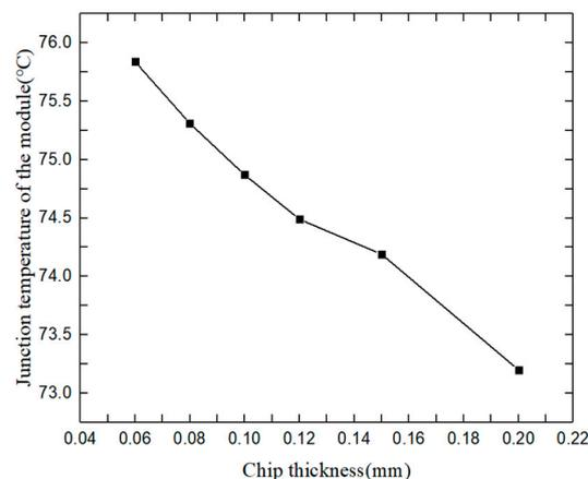
**Figure 4.** Junction temperature vs. chip thickness.
