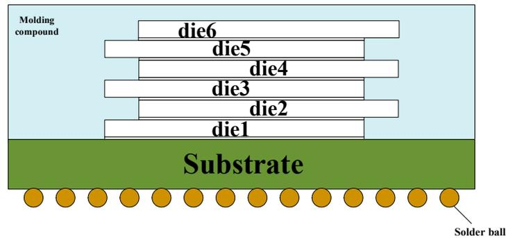
Figure 11. Schematic diagram of a six-layer stagger-stacked DDR module.
