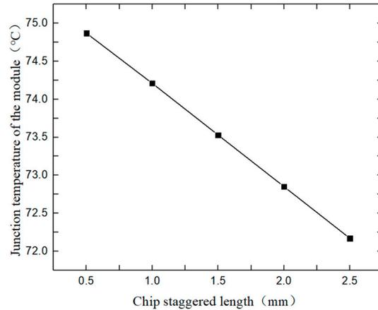
Figure 5. Junction temperature vs. chip staggered length.
