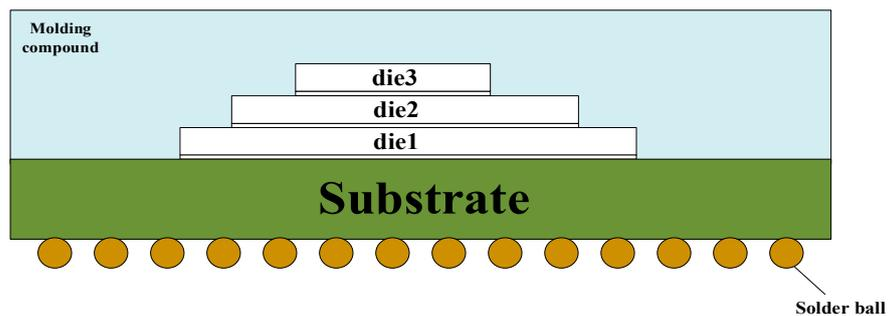
Figure 16. Schematic diagram of a three-layer pyramid package.
