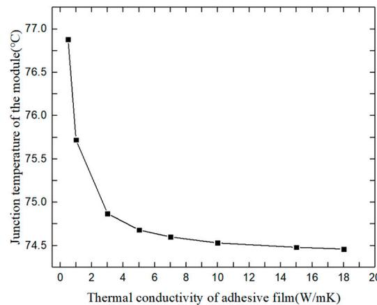
Figure 8. Junction temperature vs. thermal conductivity of adhesive film.
