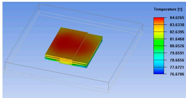
Figure 15. Optimal temperature distribution of six-layer stagger-stacked DDR module.
