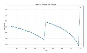
**Figure 3.** Visualization of the reward function over time, showing non-linear penalty function, reinforcing optimal path planning, and highlighting jumps from rewards per gate passed and episode completion.
