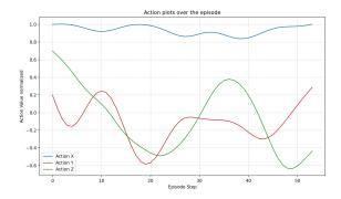
**Figure 8.** 'Action plots over the episode', which illustrates the normalized action values across the episode steps for the X (blue), Y (green), and Z (red) axes, offering insights into the control strategy of the drone's trajectory during navigation. The values reported here are normalized between 1 and -1, with 1 indicating movement in the positive direction of the axis and -1 indicating movement in the negative direction.
