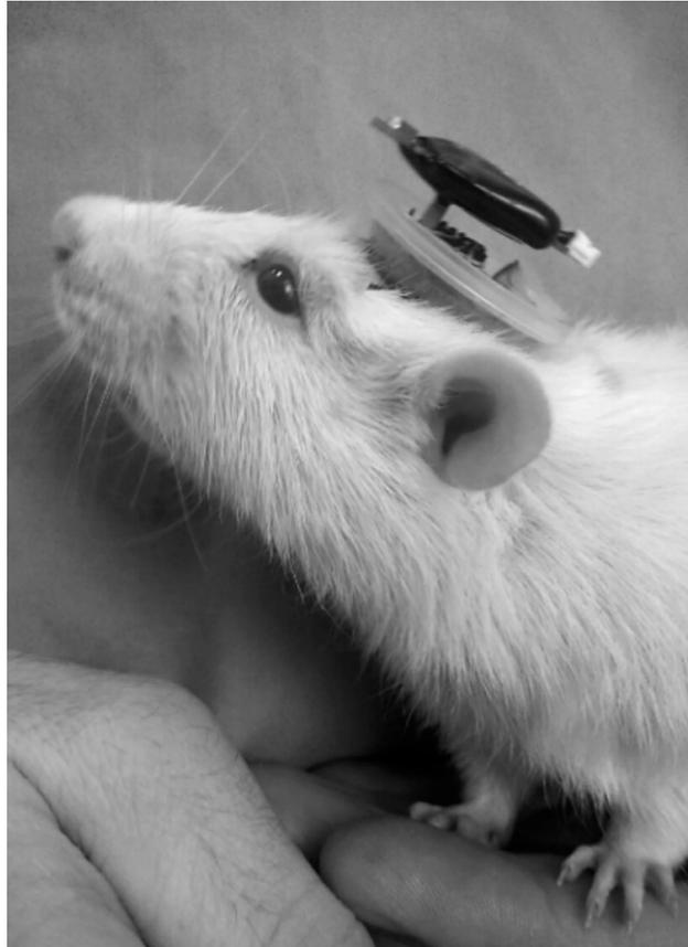
**Figure 3.** Appearance of the head-mounted transmitter in a rat during the preliminary stages of technique evaluation.
