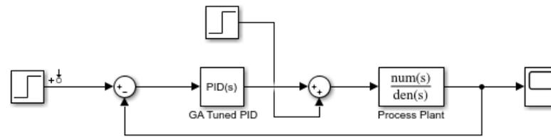
**Figure 1.** GA tuning PID control system of the wind tunnel flow field.
