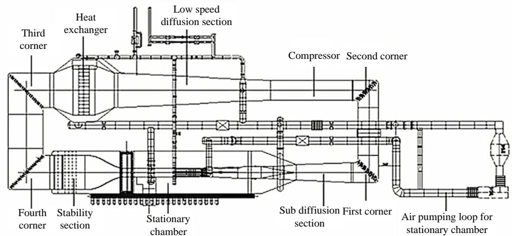
**Figure 2.** Structure of the wind tunnel system.
