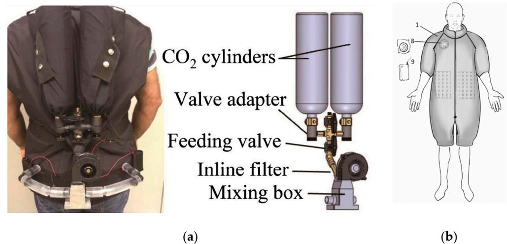
**Figure 5.** (a) Duct-type air-cooling clothing [23]; (b) Fan-type hybrid dry ice and air-cooling clothing [25].
