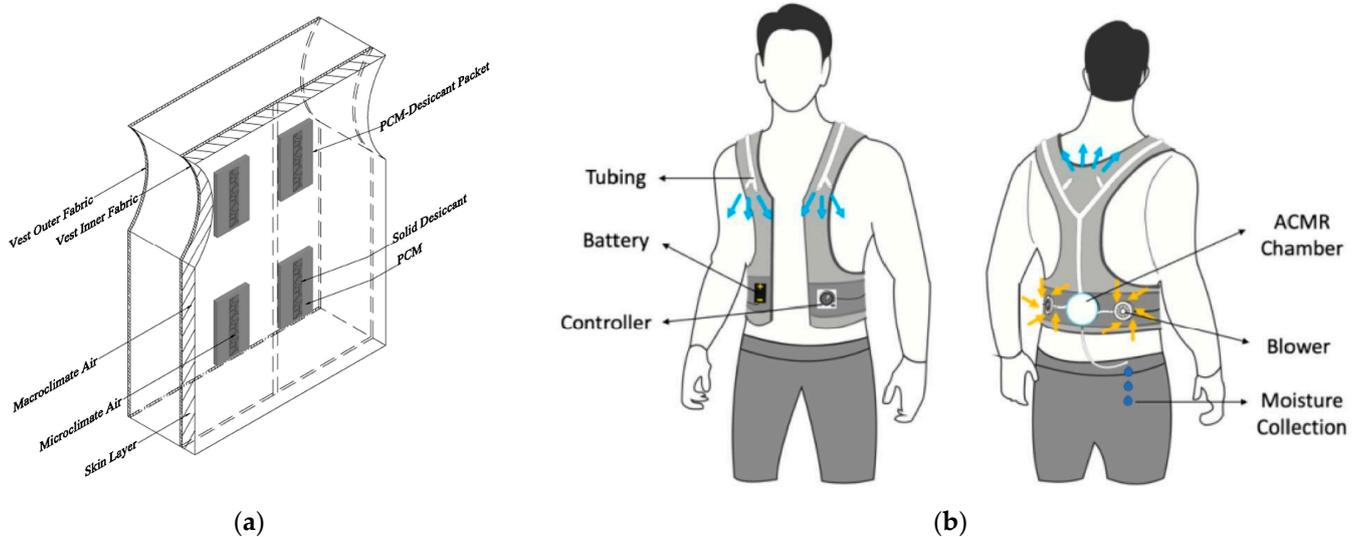
**Figure 12.** Schematic diagram of (a) PCM composite desiccant packages [89] and (b) ACMR for clothing [72].
