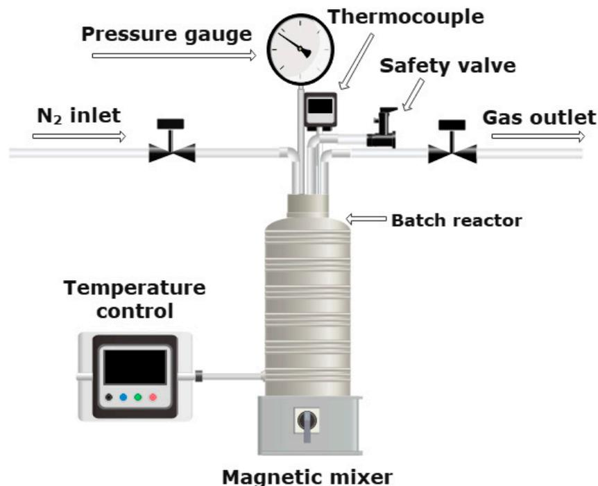
**Figure 1.** Scheme of apparatus for batch SWE.
