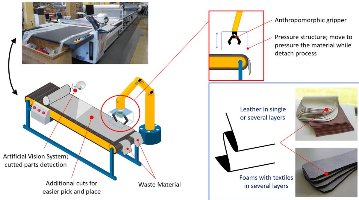
**Figure 6.** Detach using press and grasp, applied for human-oriented design of collaborative robots in leather-cutting process.
