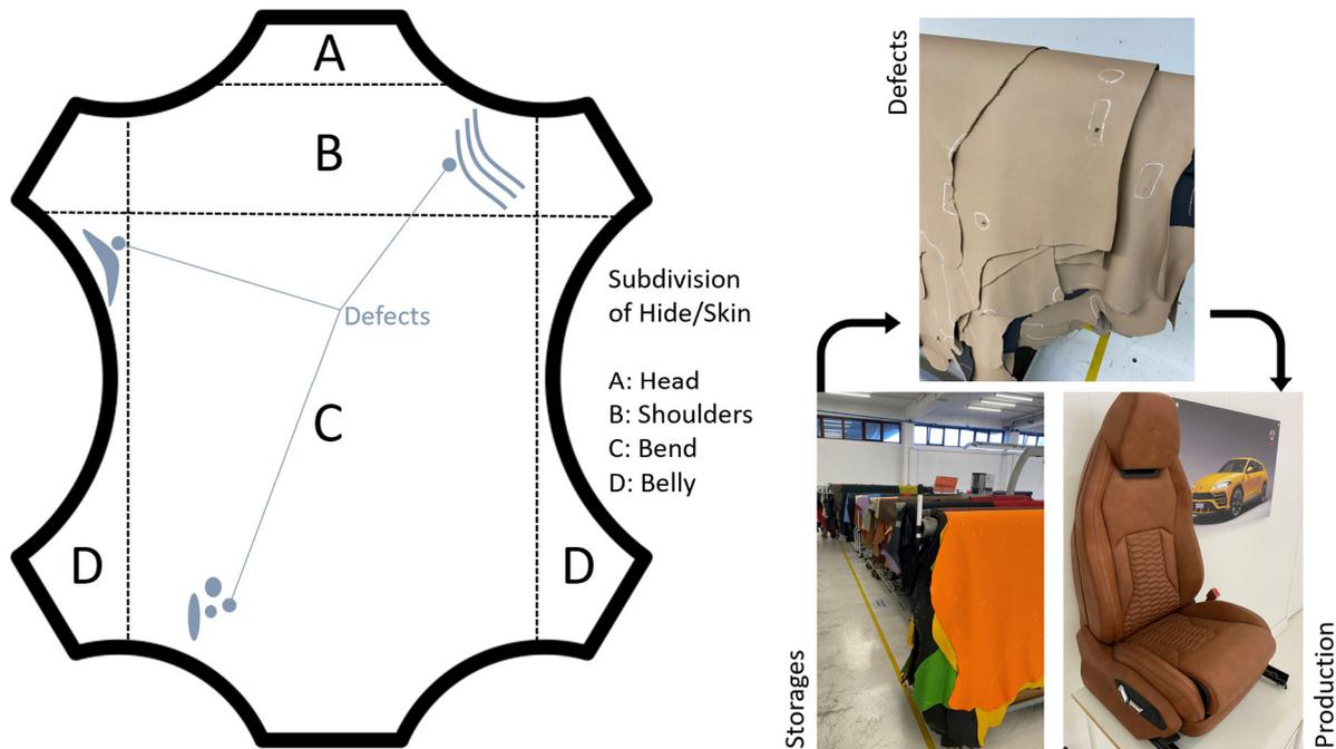
**Figure 7.** Leather defect detection and classification importance. Visual inspection methods by humans in the beginning can be replaced by HRC and RFID during the process. These effects occur due to different reasons, e.g., raw hides and animal wounds, damage during transport, moisture, folds, wrinkles, and dirt.
