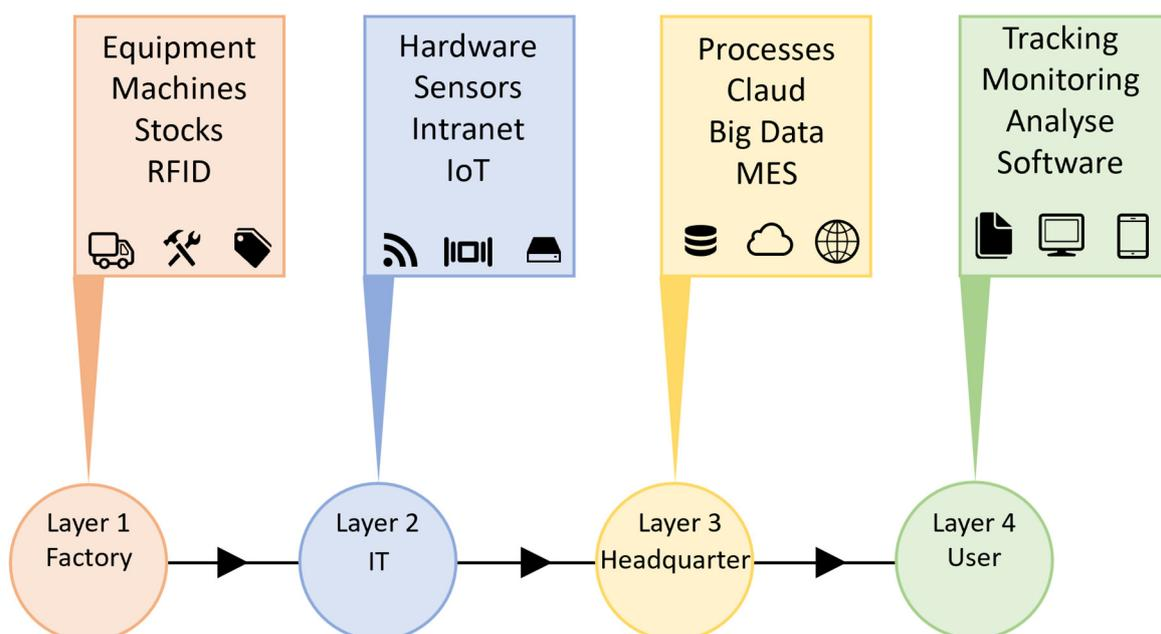
**Figure 5.** Radio frequency identification (RFID) configuration for manufacturing execution system (MES) processing.
