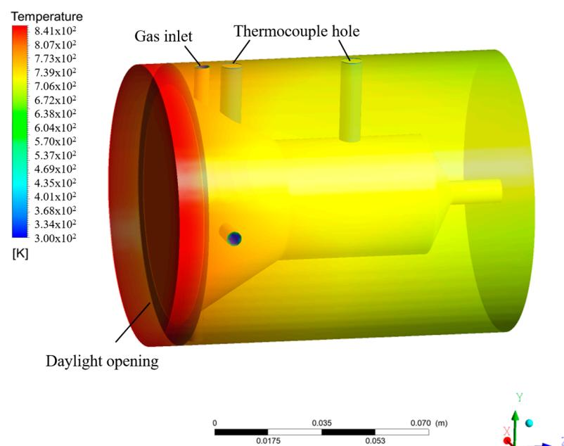
**Figure 1.** Temperature distribution contour map of solar reactor.
