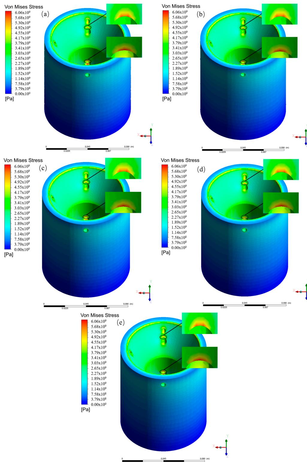
**Figure 11.** Thermal stress clouds of the reactor under different inlet velocities. **(a)** The inlet velocity is 0.003 m/s; **(b)** the inlet velocity is 0.015 m/s; **(c)** the inlet velocity is 0.03 m/s; **(d)** the inlet velocity is 0.06 m/s; **(e)** the inlet velocity is 0.09 m/s.
