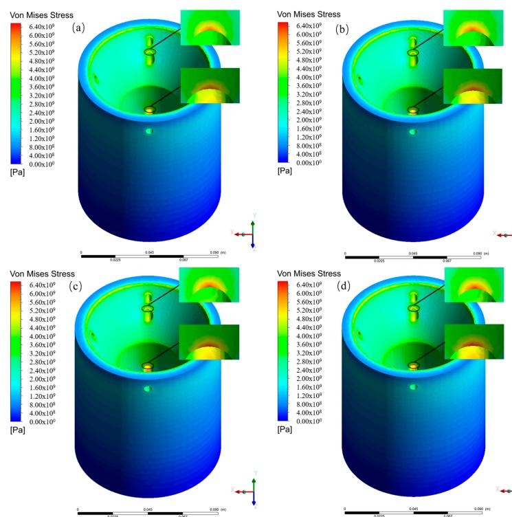
**Figure 9.** Thermal stress cloud diagrams under different reactor inner wall emissivities. (a) The emissivity is 0.2; (b) the emissivity is 0.3; (c) the emissivity is 0.4; (d) the emissivity is 0.5.
