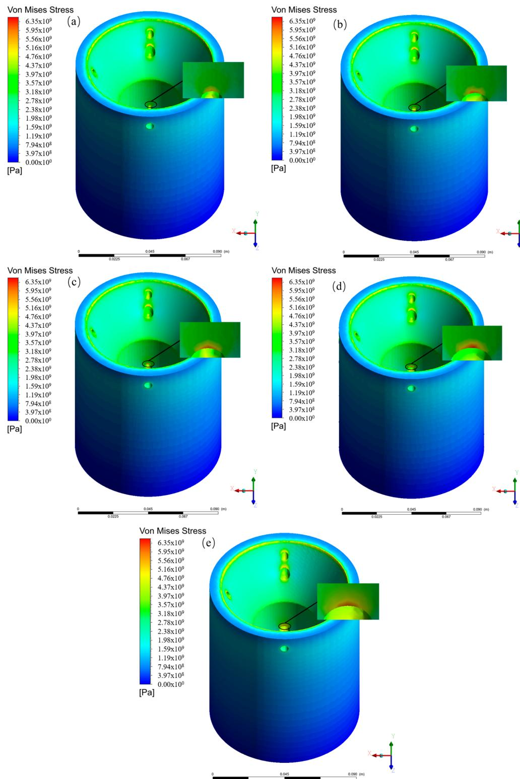
**Figure 15.** Thermal stress cloud diagrams of reactors with different thermocouple diameters. **(a)** The thermocouple diameter is 3 mm; **(b)** the thermocouple diameter is 4 mm; **(c)** the thermocouple diameter is 5 mm; **(d)** the thermocouple diameter is 6 mm; **(e)** the thermocouple diameter is 7 mm.
