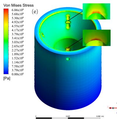
**Figure 13.** Thermal stress clouds of the reactor under different working pressures. (a) The working pressure is 0.1 MPa; (b) the working pressure is 0.5 MPa; (c) the working pressure is 1 MPa; (d) the working pressure is 1.5 MPa; (e) the working pressure is 2 MPa.
