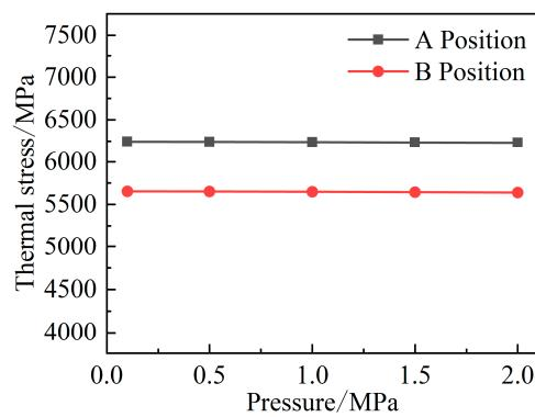
Figure 12. Influence of working pressure on thermal stress.
