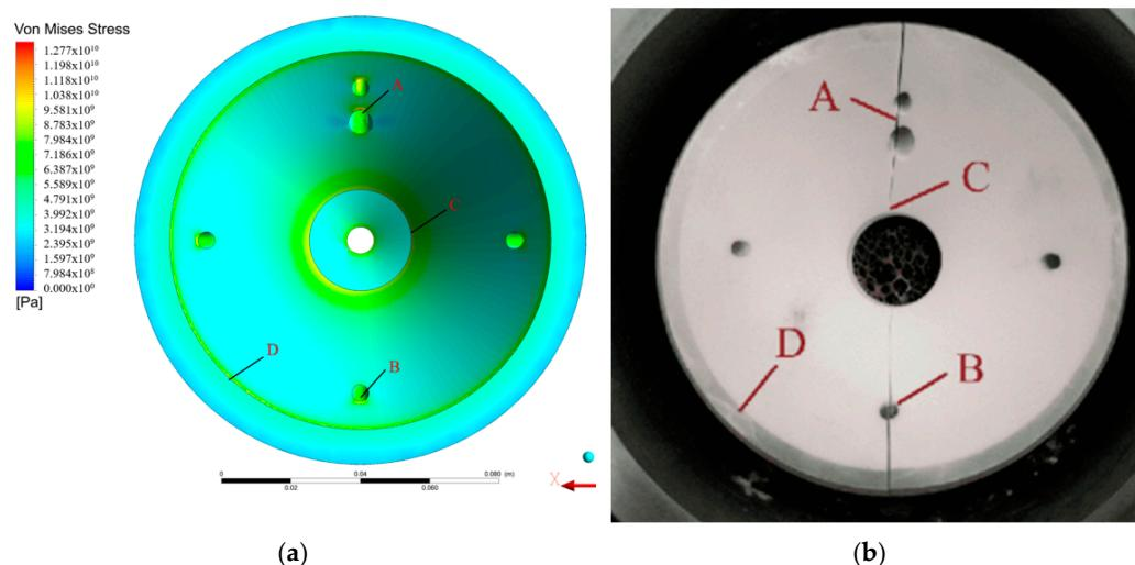
**Figure 4.** The simulation results are compared with the literature. (a) Von Mises stress simulation results; (b) experimental results in the literature. (A: the inlet opening, B: the front thermocouple opening, C: aperture, D: the lighting opening).
