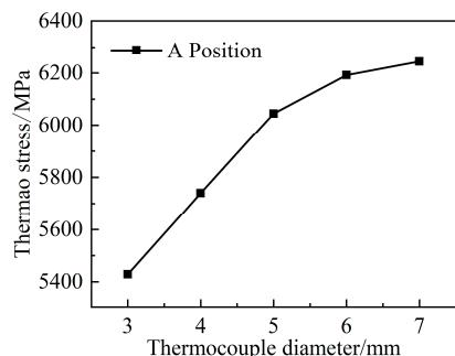
**Figure 14.** Influence of thermocouple diameter on thermal stress.
