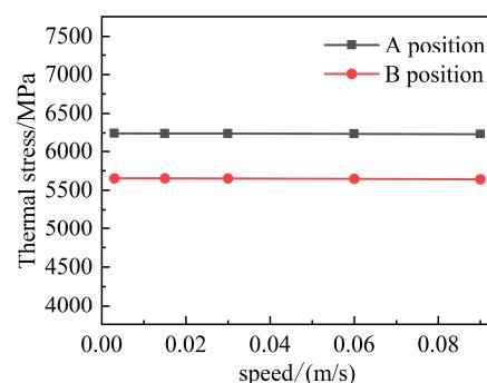
**Figure 10.** Effect of inlet velocity on thermal stress.
