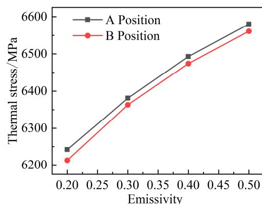
**Figure 8.** The influence of the emissivity of the reactor's inner wall material on thermal stress.
