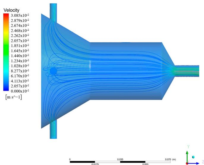
**Figure 2.** Velocity distribution contour map of solar reactor.
