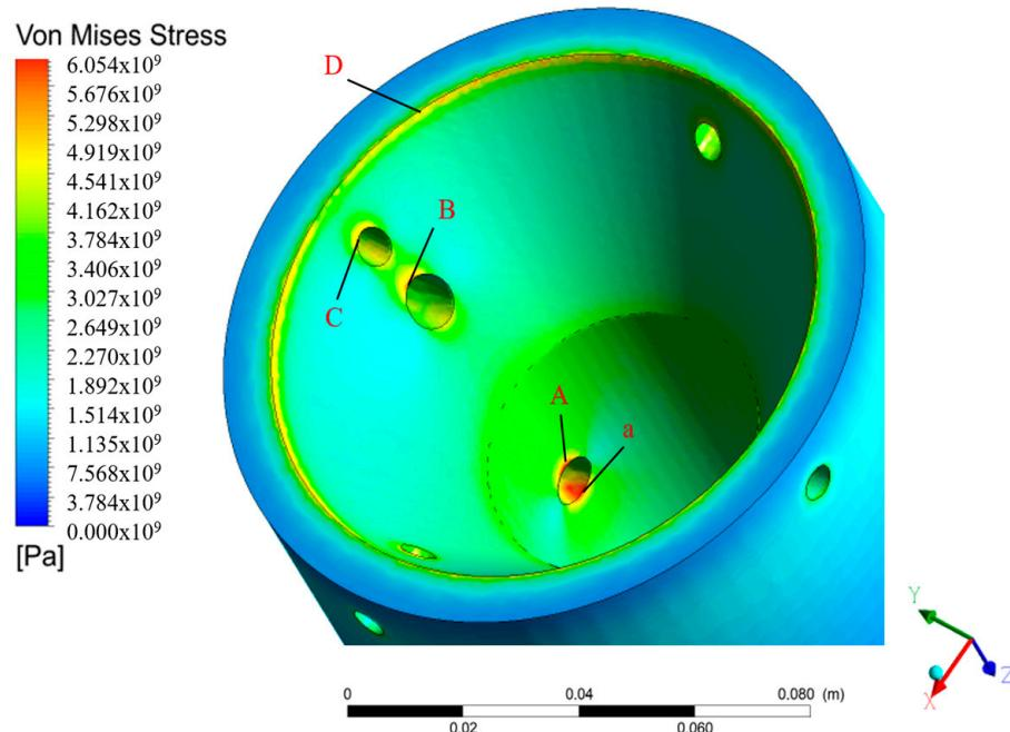
**Figure 5.** Thermal stress distribution cloud. (A, a: the thermocouple opening, B: the front thermocouple opening, C: the inlet opening, D: the lighting opening).
