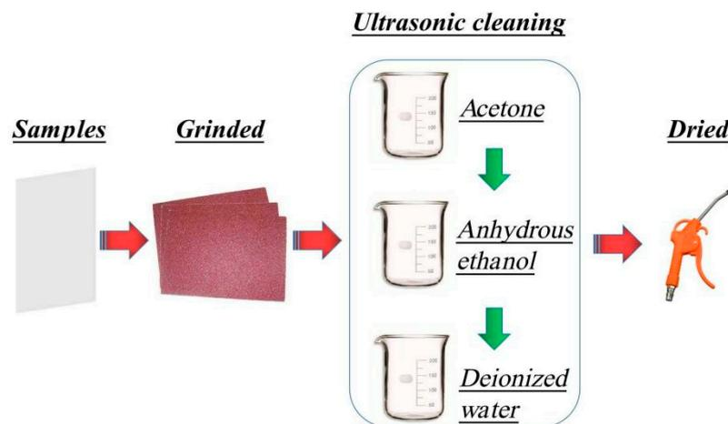
Figure 1. Nickel sample preparation processes.
