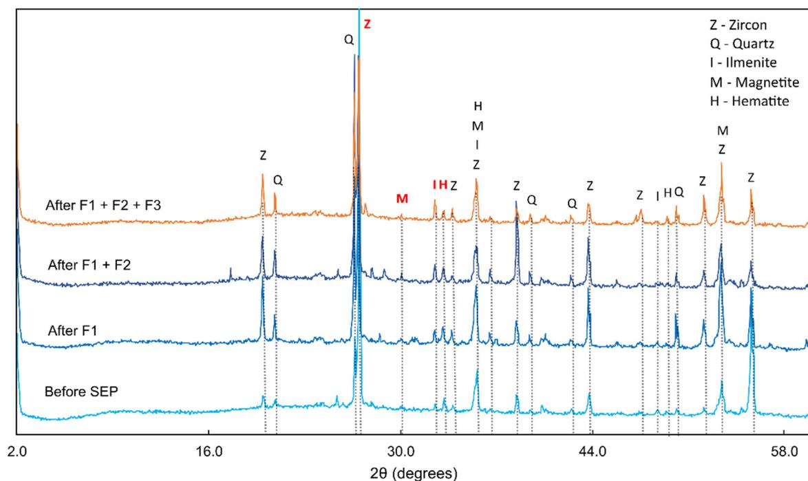
**Figure 1.** X-ray diffractogram of tailings sample before and after each step of the SEP. The peaks cited in the discussion are represented in red letters:  $d$  = 2.70 Å (hematite),  $d$  = 2.76 Å (ilmenite),  $d$  = 2.97 Å (magnetite), and  $d$  = 3.31 Å (zircon).
