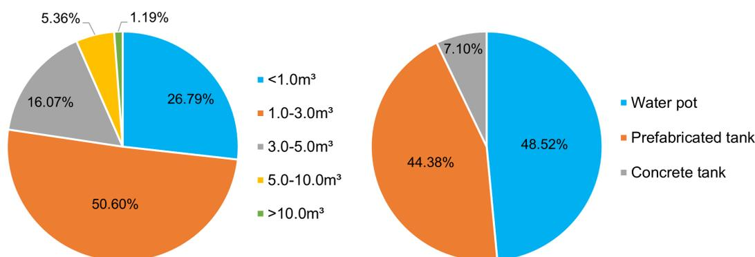
**Figure 6.** Characteristics of rainwater tanks in terms of capacity (left) and materials (right).
