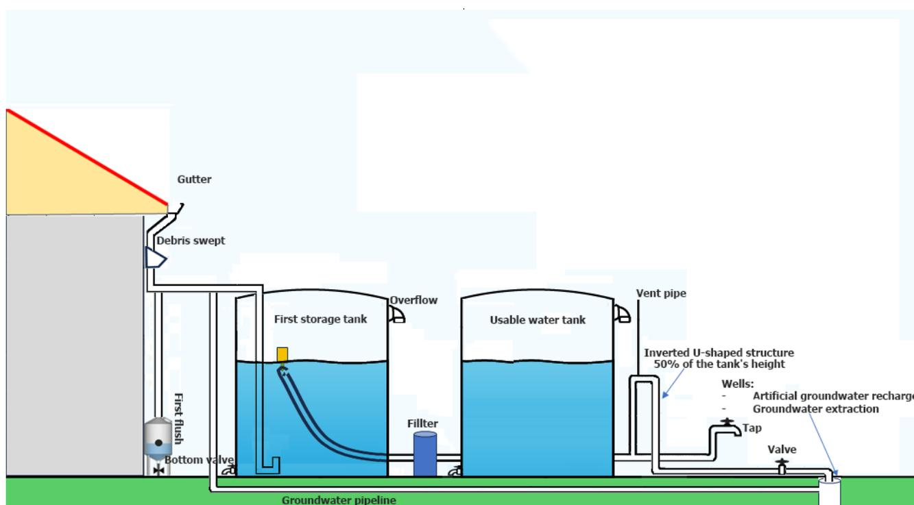
**Figure 2.** Rainwater harvesting system developed in the study, including artificial groundwater recharge and groundwater extraction, adopted from the website <https://content.ces.ncsu.edu/mosquito-control-for-rainwater-harvesting-systems> assessed on 31 December 2021.
