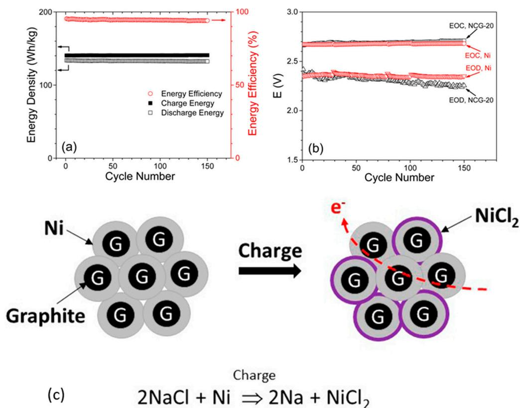
**Figure 3.** (a) Energy efficiency and energy densities of NCG cell. (b) Voltage plots of end of charge and end of discharge for NCG (black) and Ni cathode (red) at 190 °C, respectively. (c) Schematic view of the nickel-carbon core-shell microstructure NCG. Reprinted with permission from [54]. Copyright 2017, American Chemical Society.
