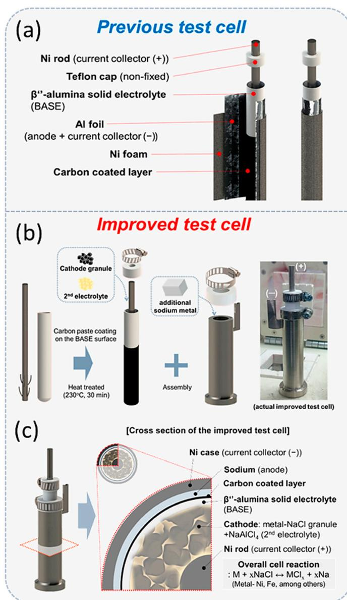
**Figure 18.** (a) Structure of previous test cell, (b) assembly process and improved cell and (c) cross-section of improved test cell. Reprinted from [200] under terms of Creative Commons Attribution (CC BY 4.0) license (<https://creativecommons.org/licenses/by/4.0/> accessed on 15 September 2023). Copyright 2022; B.-M. Ahn, C.-W. Ahn, B.-D. Hahn, J.-J. Choi, Y.-D. Kim, S.-K. Lim and J.-H. Choi; published by MDPI.
