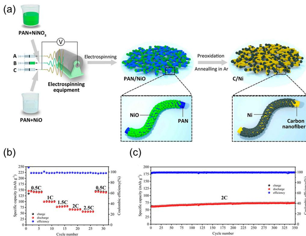
**Figure 4.** (a) Schematic diagram of the synthesis process of the nickel–carbon nanofibers. (b) Performance of the nickel–carbon cathode at different rates. (c) Cycle performance of the nickel–carbon cathode at 2C. Reprinted with permission from [74]. Copyright 2020, American Chemical Society.
