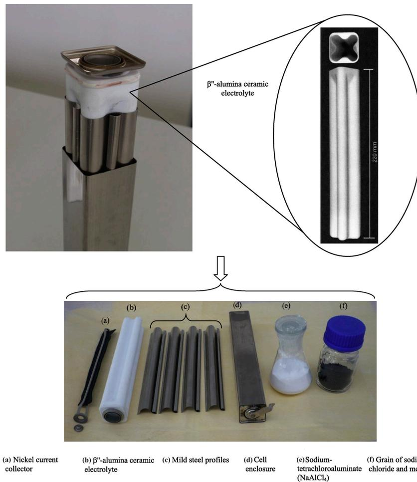
**Figure 12.** Constructional elements of current commercial Na-NiCl<sub>2</sub> cell. Reprinted from [15], copyright 2015, with permission from Elsevier.
