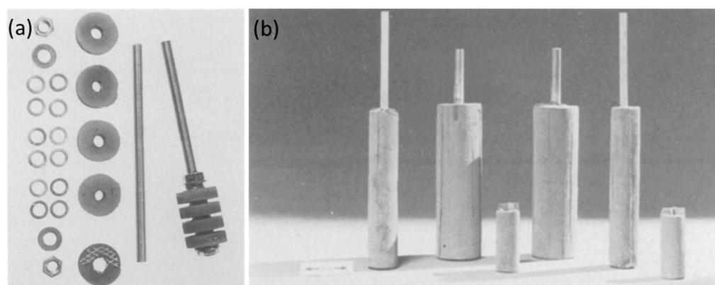
**Figure 10.** (a) Porous iron disk and (b) solid-cylinder cathode design proposed for the first generation of ZEBRA cell. Used with permission of IOP Publishing, Ltd., from [56], copyright 1987, permission conveyed through Copyright Clearance Center, Inc.
