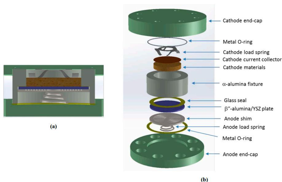
**Figure 20.** (a) Schematic view of an assembled prototypal planar Na-NiCl<sub>2</sub> cell; (b) expanded view of each element. Reprinted from [46], under terms of Creative Commons Attribution (CC BY 4.0) license (<https://creativecommons.org/licenses/by/4.0/> accessed on 15 September 2023). Copyright 2016; G. Li, X. Lu, J.Y. Kim, K.D. Meinhardt, H.J. Chang, N.L. Canfield and V.L. Sprenkle; published by Nature Communications.
