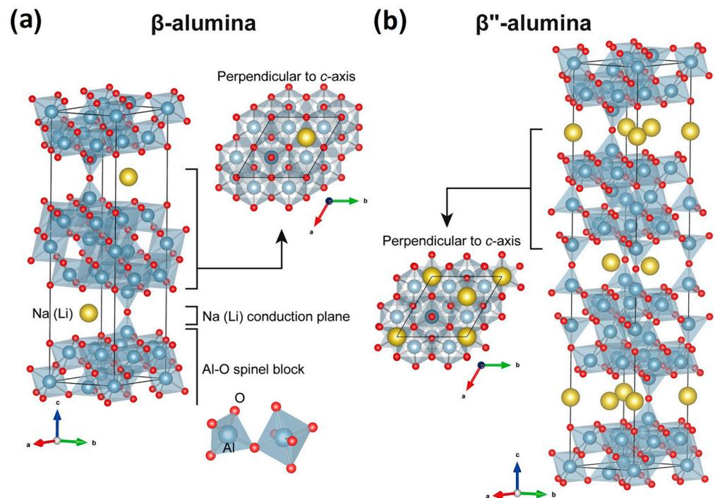
**Figure 5.** Crystal structures of (a) Na-β-Al<sub>2</sub>O<sub>3</sub> and (b) Na-β''-Al<sub>2</sub>O<sub>3</sub>. Reprinted from [80], copyright 2017, with permission from Elsevier.
