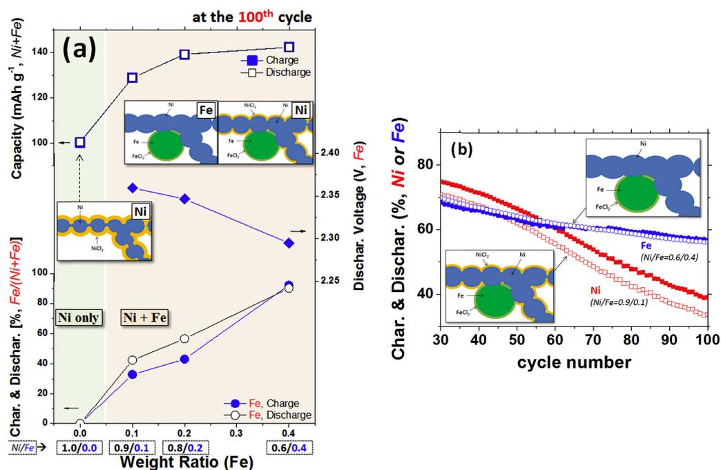
**Figure 2.** (a) Variations in Fe capacities, discharge voltages (Fe) and total capacities (Ni+Fe) with Fe amount in Na-NiCl<sub>2</sub> cell and Na-(Ni,Fe)Cl<sub>2</sub> cells (at the 100th cycle) and (b) cycle performances of Fe (0.6/0.4 cell) and Ni (0.9/0.1 cell) in Na-(Ni,Fe)Cl<sub>2</sub> cells. Reprinted from [59], copyright 2016, with permission from Elsevier.
