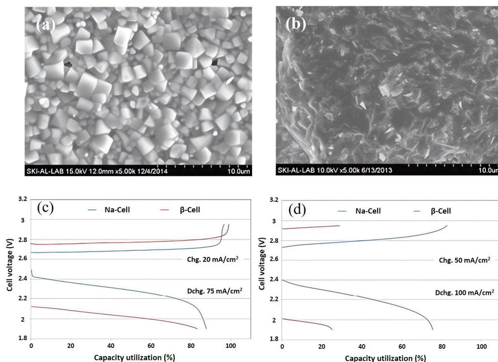
**Figure 8.** SEM images of the (a) surface and (b) cross-section of the NaSICON ceramic. Charge and discharge profiles for prototype cells with 9.7 Ah capacities at 195 °C during (c) charge at 20 mA cm<sup>-2</sup>–discharge at 75 mA cm<sup>-2</sup> and (d) charge at 50 mA cm<sup>-2</sup>–discharge at 100 mA cm<sup>-2</sup>. Reprinted from [37], copyright 2015, with permission from Elsevier.
