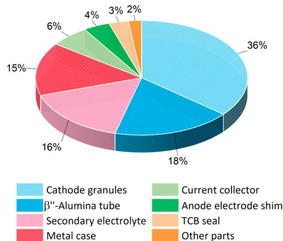
**Figure 13.** Weight distribution of components in a typical commercial Na-NiCl<sub>2</sub> cell.
