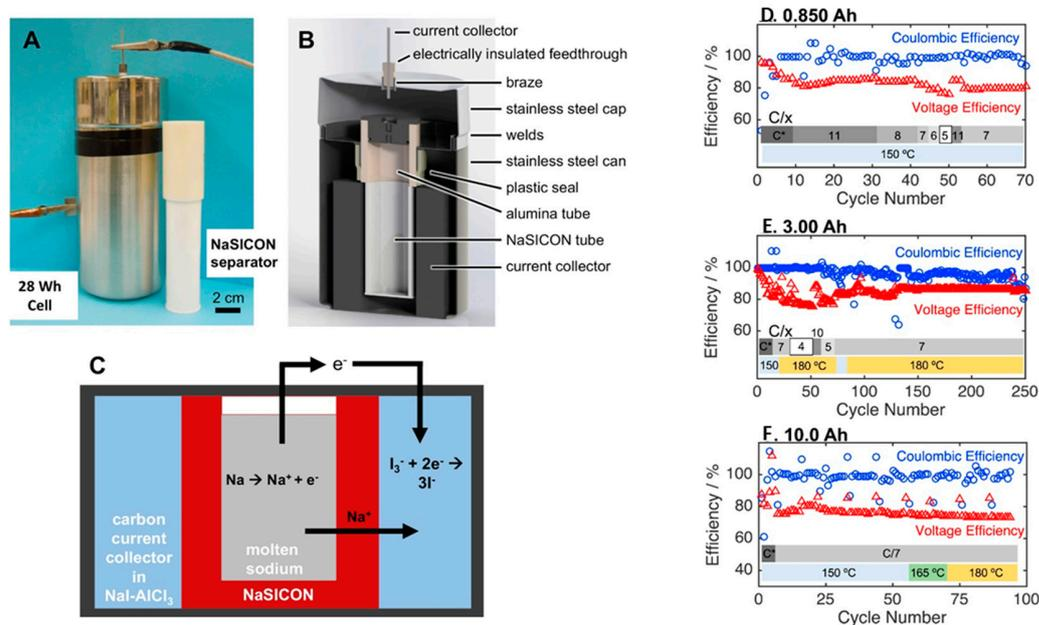
**Figure 9.** (A) Photograph of prototype 28 Wh (10 Ah) NaI battery assembly with NaSICON separator at right. (B) A 3D model of the 28 Wh NaI battery assembly. (C) Schematic of battery depicting chemical reactions and ion movement during battery discharge. Coulombic efficiency, voltage efficiency, operating temperature and discharge rate for NaI batteries of different sizes: (D) 0.850 Ah, (E) 3.00 Ah, (F) 10.0 Ah. Reprinted from [166], copyright 2017, with permission from Elsevier.
