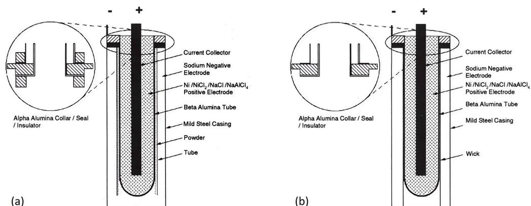
**Figure 11.** (a) First generation and (b) second generation of the tubular ZEBRA cell. Used with permission of SAE International, from [177], copyright 1991, permission conveyed through Copyright Clearance Center, Inc.
