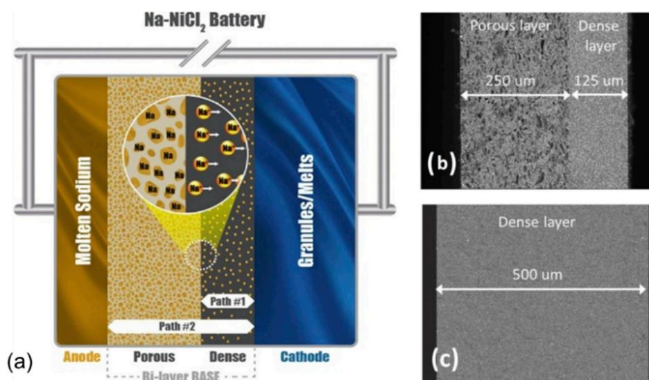
**Figure 6.** (a) A schematic view of the Na-NiCl<sub>2</sub> battery with bi-layer BASE. SEM images of (b) the bi-layer BASE and (c) standard dense BASE. Reprinted from [90], copyright 2018, with permission from Elsevier.
