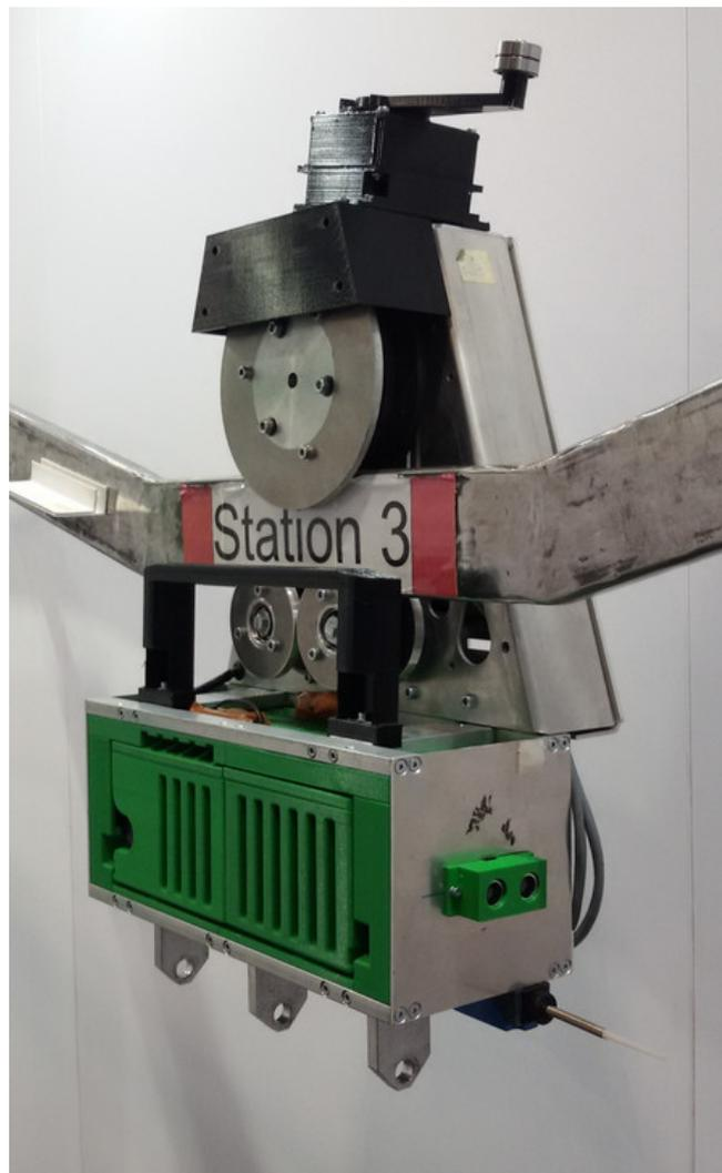
**Figure 3.** Battery-powered test trolley with single load-bearing wheel and support wheel for turnout functionality on the top [14].
