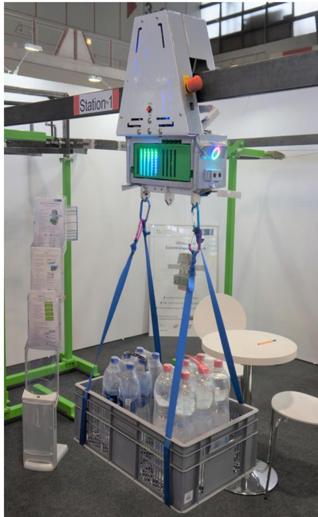
**Figure 4.** Test trolley with 20 kg load on rectangular profile track [14].
