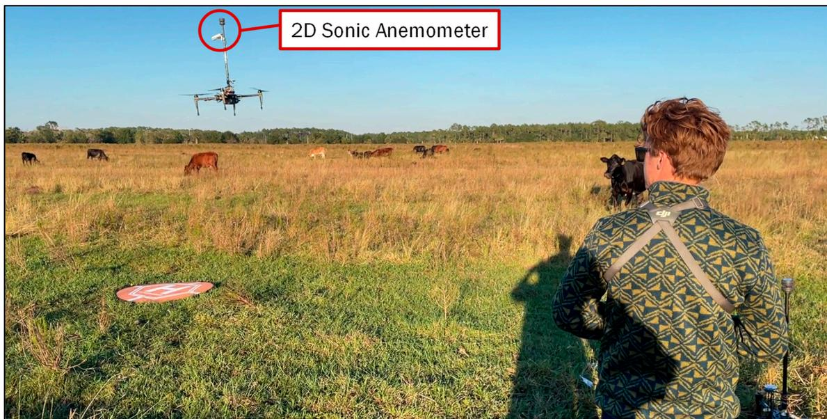
**Figure 26.** Instrumented multi-rotor vehicle in flight under manual control.
