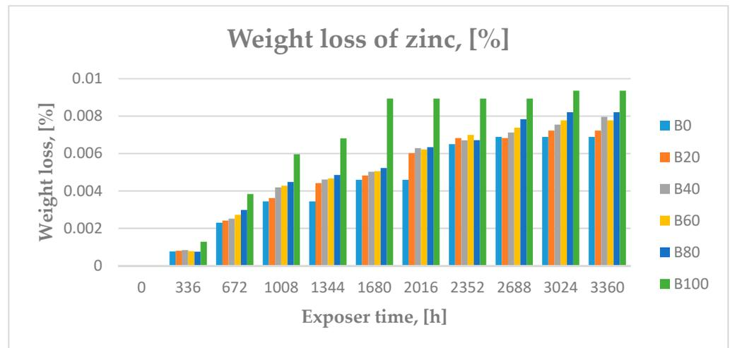
Figure 4. Weight loss of zinc plates measured every 336 h for 3360 h, [%].
