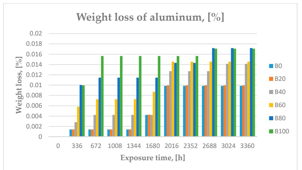
**Figure 3.** Weight loss of aluminum plates measured every 336 h for 3360 h, [%].
