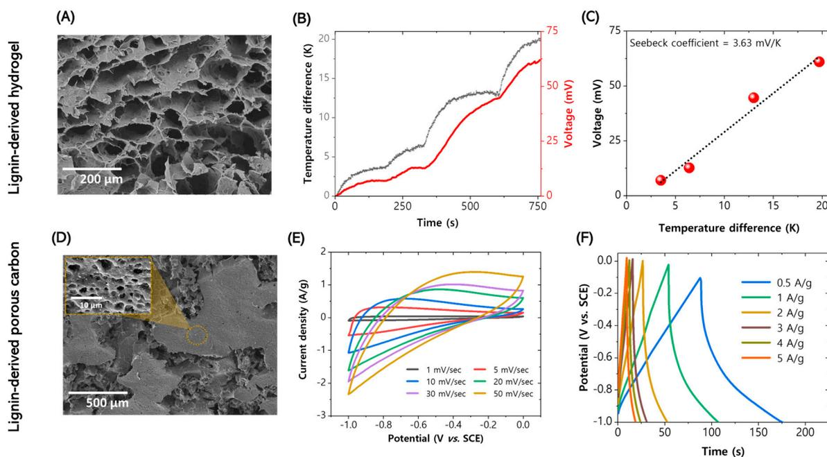
**Figure 1.** Lignin-derived hydrogel (A) morphology, (B) voltage response to axial temperature difference, and (C) Seebeck coefficient. Lignin-derived porous carbon (D) porous morphology, (E) cyclic voltammetry graphs, and (F) galvanostatic charge—discharge curves.
