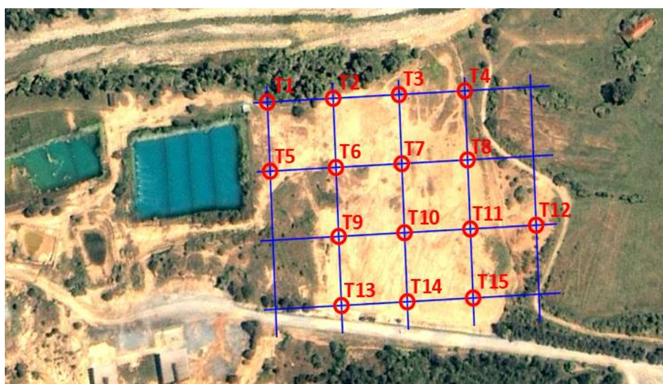
Figure 3. Soil sampling grid at the old arsenopyrites concentrate storage area (former METBA plot) before remediation.
