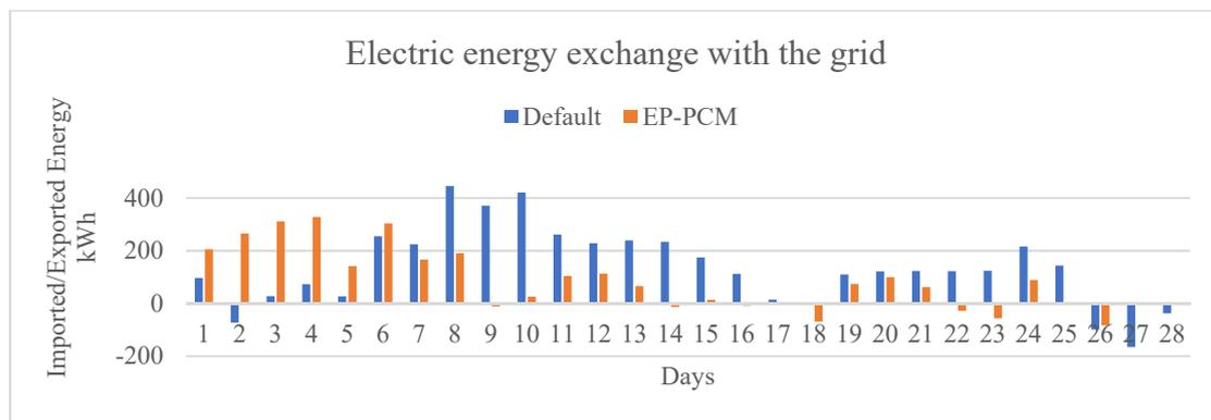
**Figure 4.** Daily electric energy exchange of nZEB Living Lab with the grid in July 2020.
