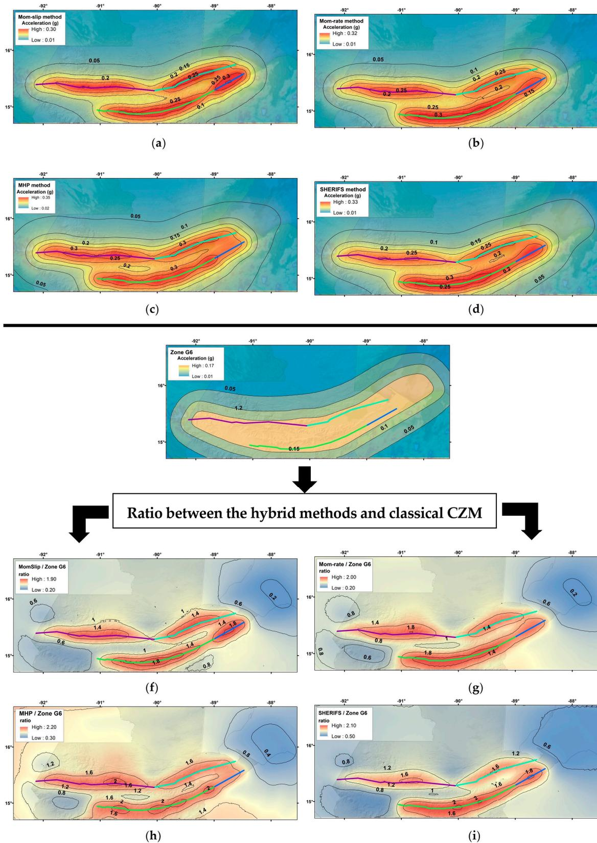
**Figure 2.** Result maps of PGA obtained using hybrid methods: (a) mom-slip, (b) mom-rate, (c) MHP, and (d) SHERIFS. (e) The map of PGA obtained using the classical zoning method (CZM) for the G6 zone. And finally, the ratio maps between the PGA value obtained with hybrid methods and the CZM method for: (f) mom-slip, (g) mom-rate, (h) MHP, and (i) SHERIFS.
