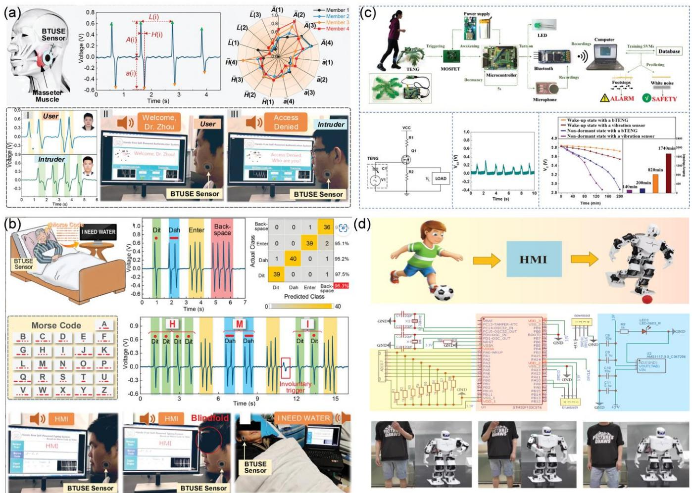
**Figure 11.** Bioinspired TENG for intelligent control. (a,b) Bionic TENG for HMI applications. Reprinted with permission from Ref. [59]. Copyright 2021, Wiley. (c) The leaf-like tentacle plant structure bionic TENG is used for system awakening. Reprinted with permission from Ref. [76]. Copyright 2020, Wiley. (d) Artificial bionic skin for multi-sensory HMI. Reprinted with permission from Ref. [62]. Copyright 2022, American Chemical Society.
