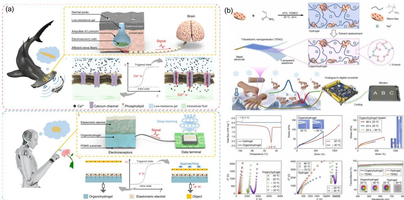
**Figure 8.** Hydrogel materials are used to construct biomimetic TENGs. (a) Bioinspired soft electroreceptors. Reprinted with permission from Ref. [4]. Copyright 2022, American Association for the Advancement of Science. (b) Antifreeze organic hydrogel TENG. Reprinted with permission from Ref. [83]. Copyright 2021, Elsevier.
