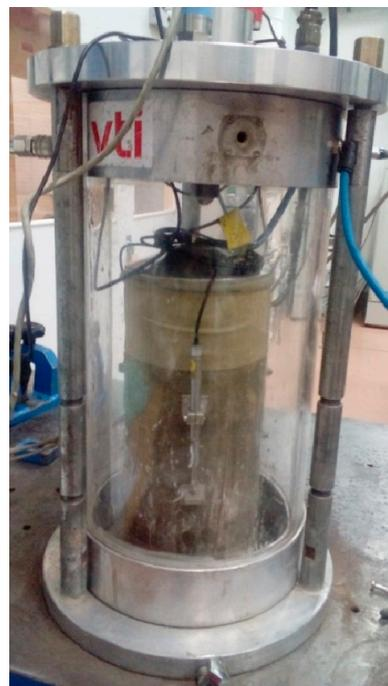
**Figure 4.** Repeated load triaxial equipment used in the study.
