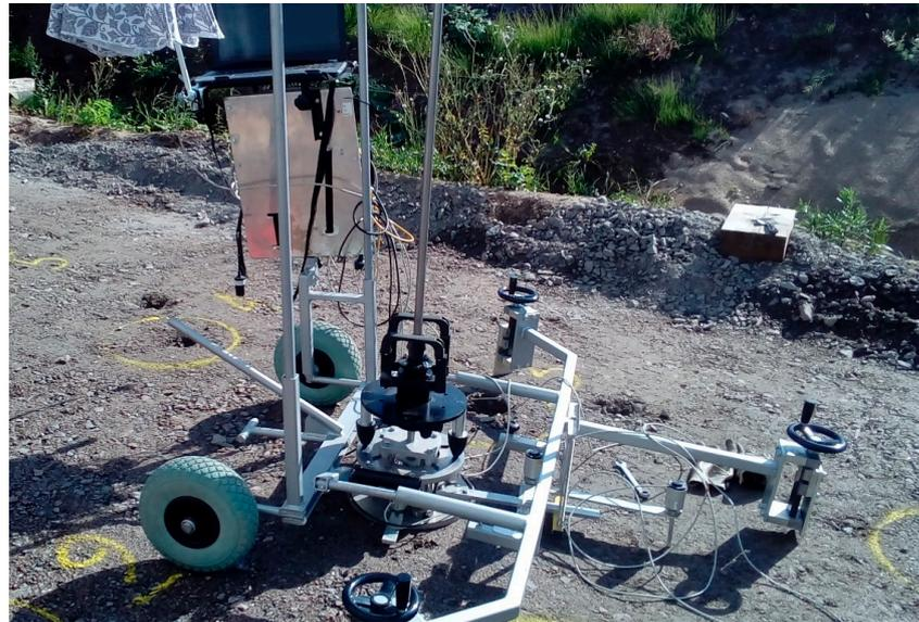
**Figure 2.** The VTI's lightweight deflectometer.
