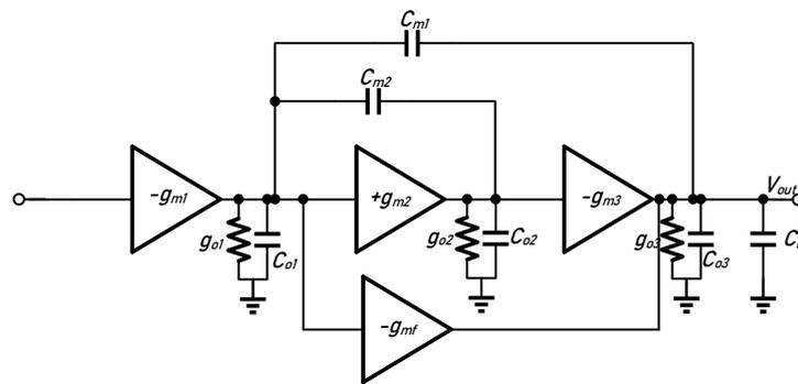
Figure 2. Topology of a three-stage *PFC* amplifier.
