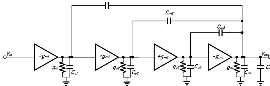
Figure 4. Topology of a four-stage multiple nested Miller compensation amplifier.
