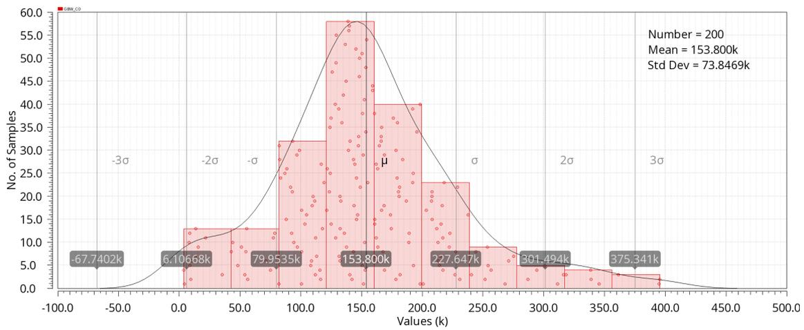
Figure 23. Histogram of GBW under 200 runs of Monte Carlo simulations with estimated parasitics.
