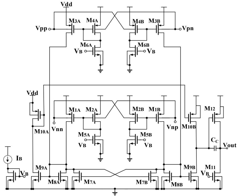
Figure 8. Bulk-driven rail-to-rail DDA circuit.
