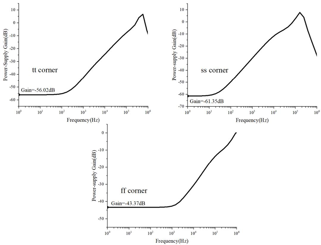
Figure 14. Power-supply gain under 50 pF load.
