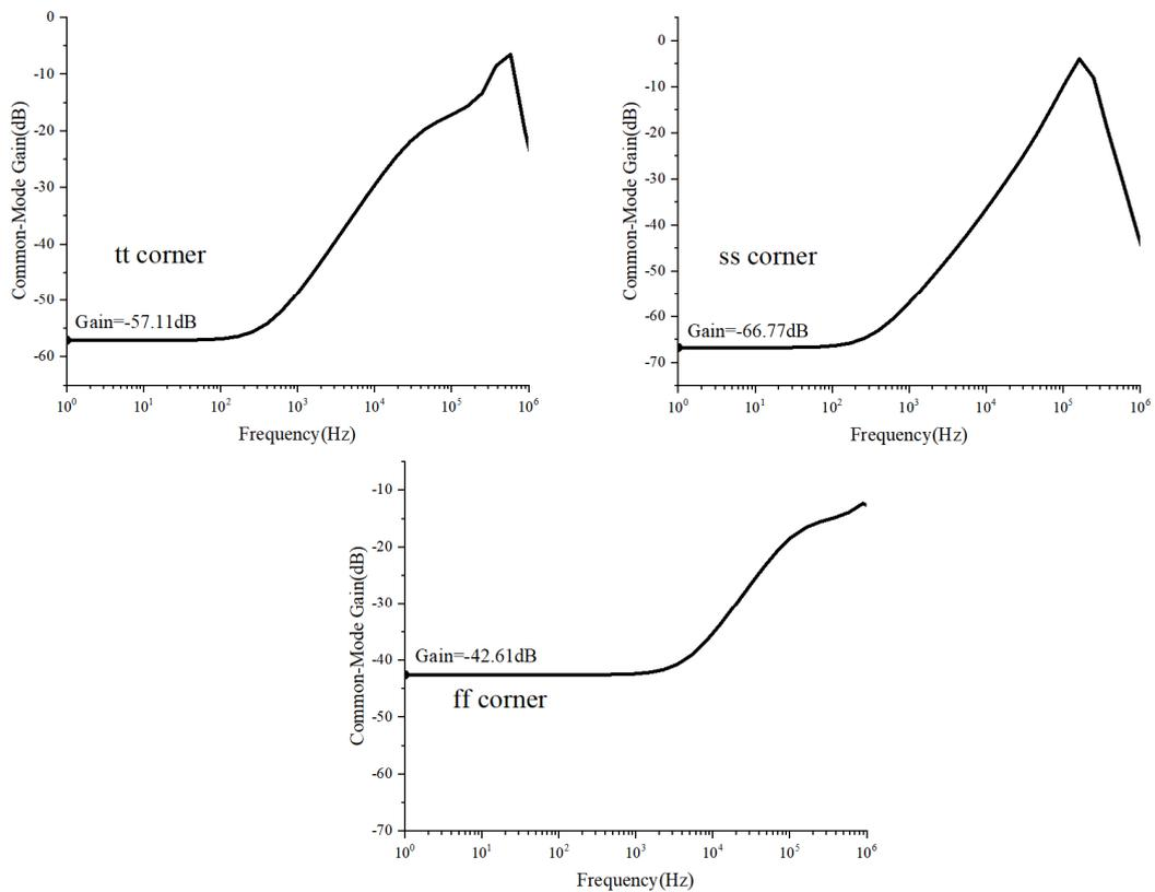
Figure 15. Common-mode gain under 50 pF load.
