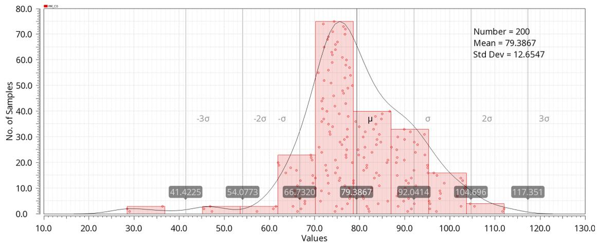
Figure 24. Histogram of PM under 200 runs of Monte Carlo simulations with estimated parasitics.
