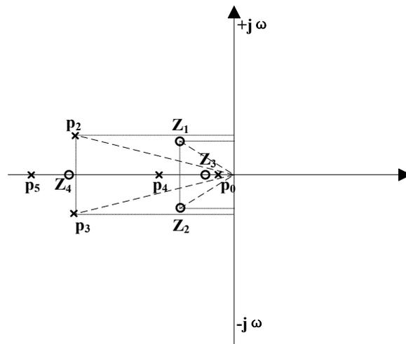
Figure 12. Pole-zero location in CFPFC op-amp.
