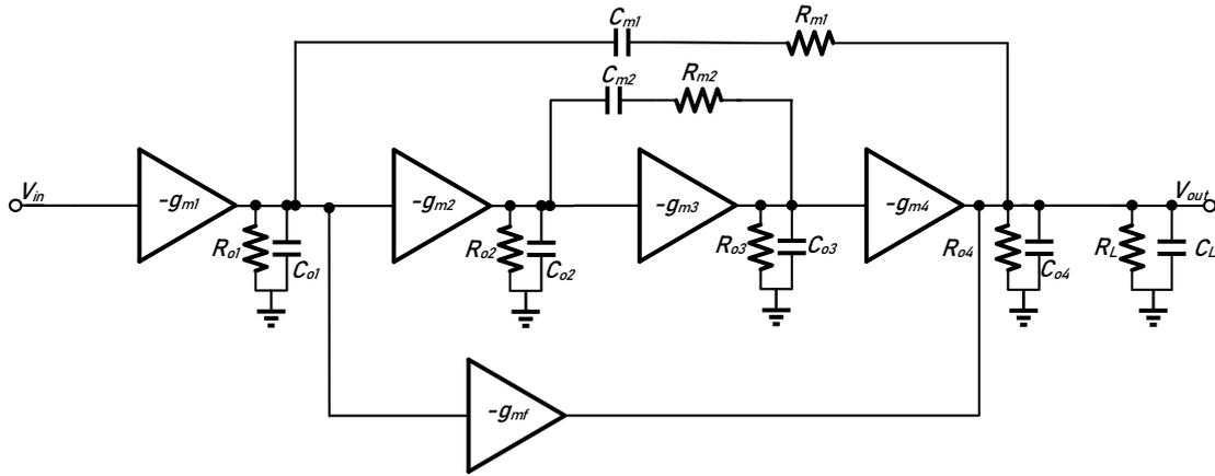
Figure 7. Topology of a four-stage SMF amplifier.
