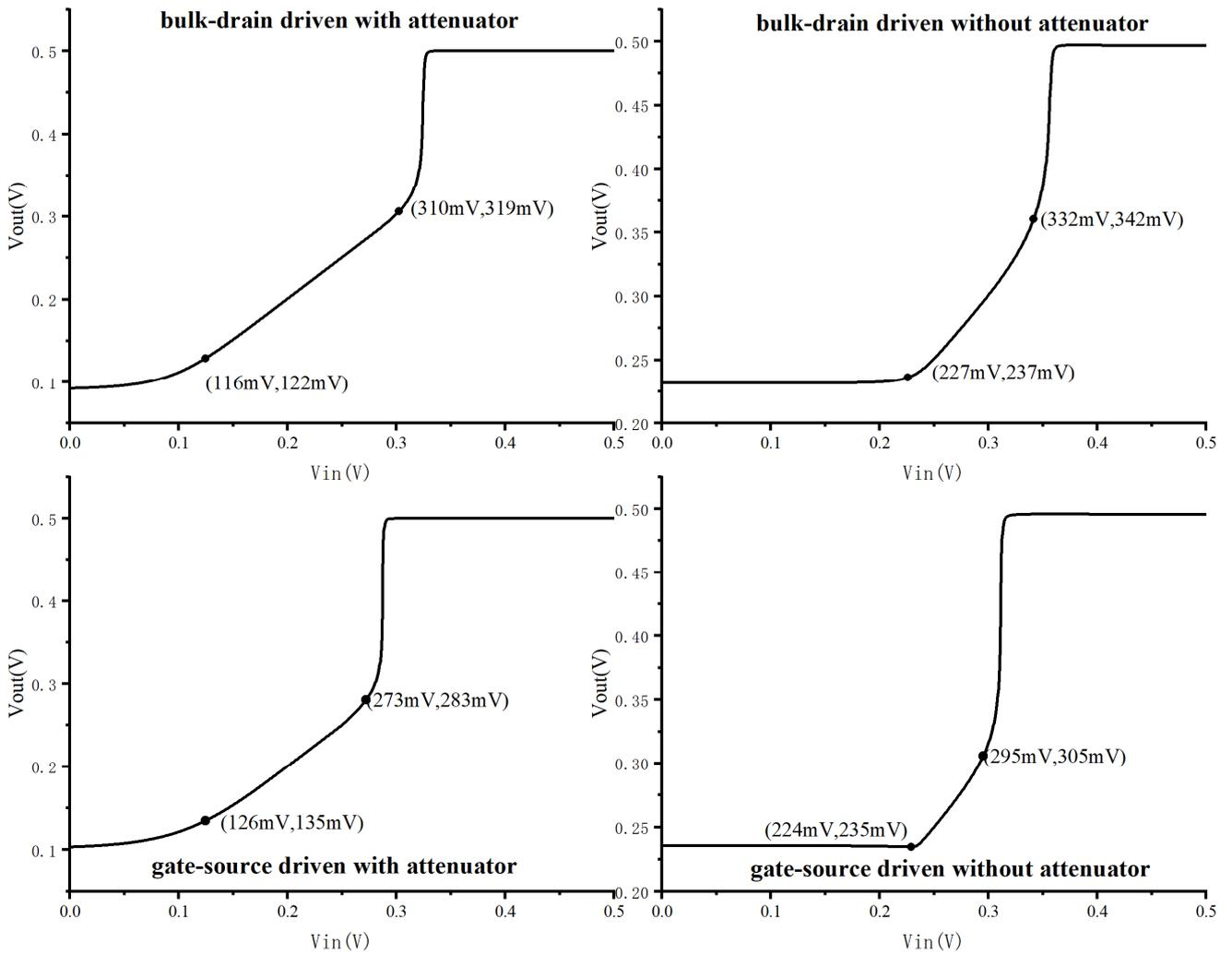
**Figure 17.** Common mode range of input and output with different input topology designs with/without low-voltage attenuator.
