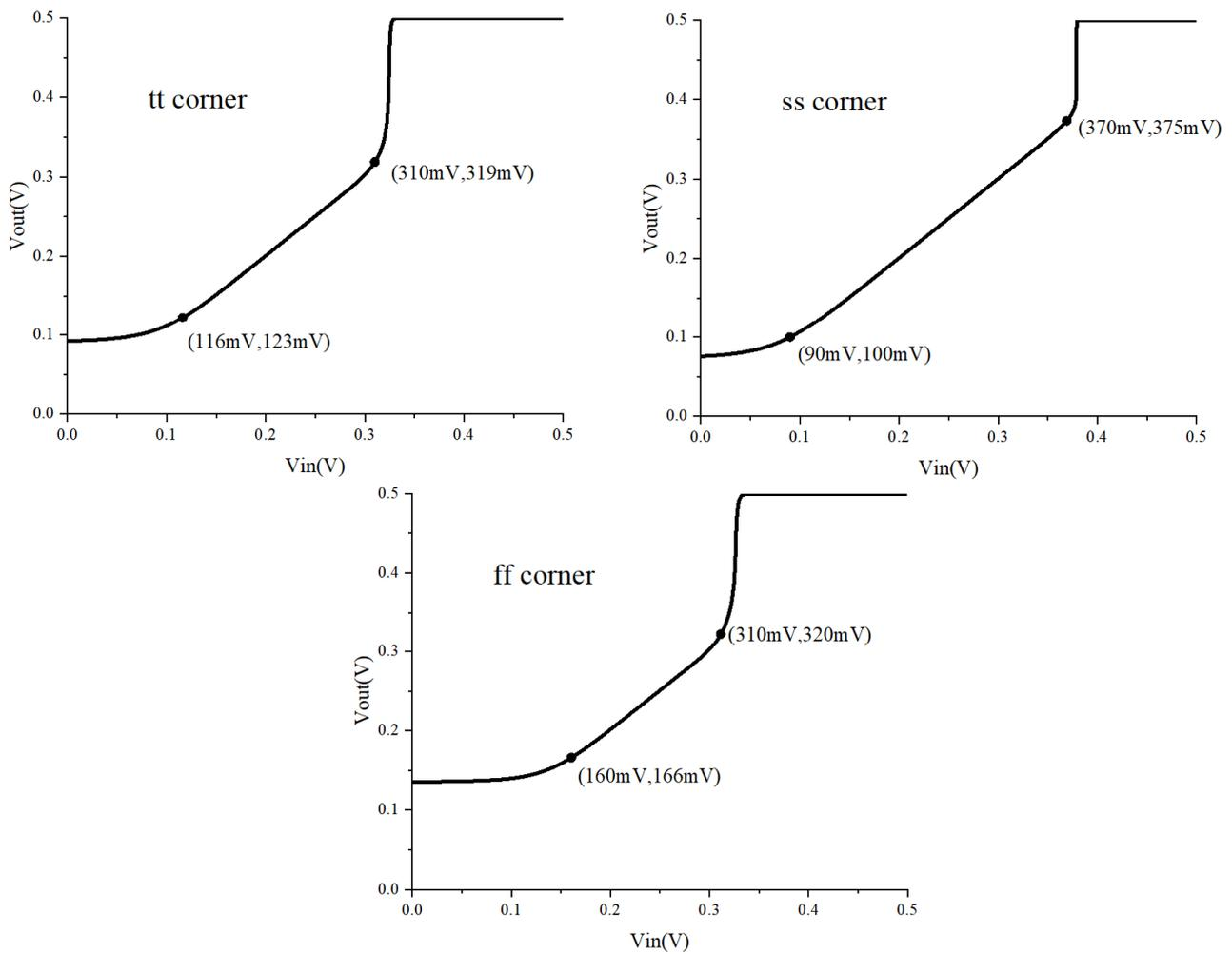
**Figure 18.** Common mode range of input and output under 50 pF load.
