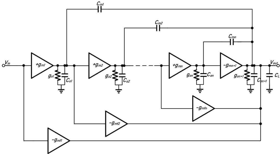
Figure 6. Topology of a four-stage NGCC amplifier.
