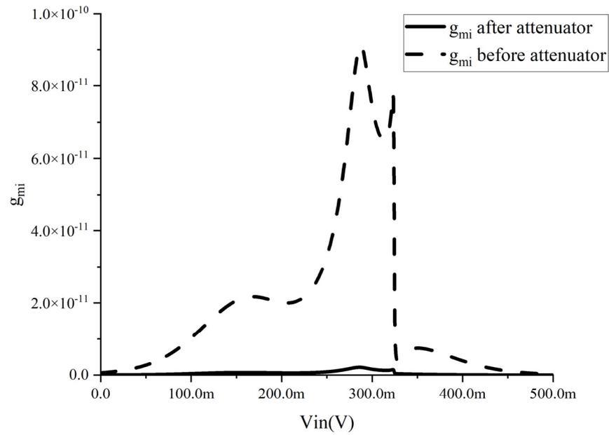
**Figure 21.** Simulation of  $g_{mi}$  against different input common-mode voltages.
