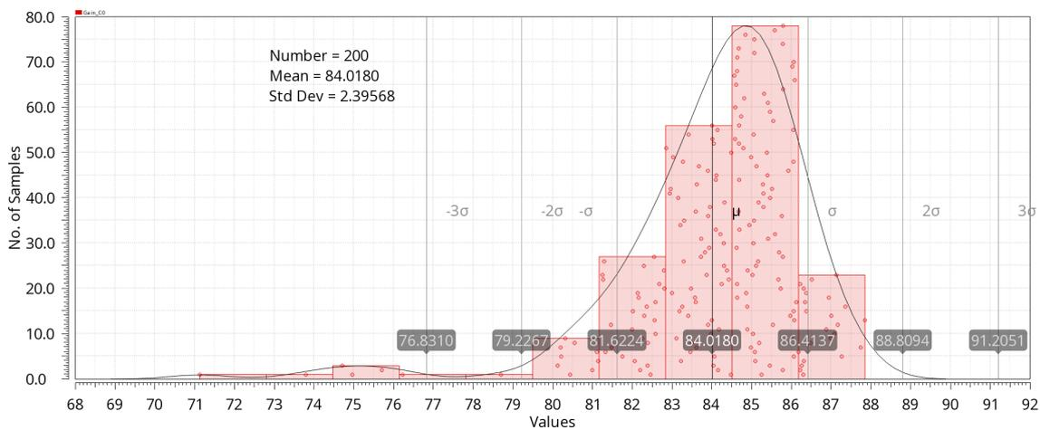
**Figure 22.** Histogram of DC gain under 200 runs of Monte Carlo simulations with estimated parasitics.
