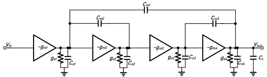
Figure 5. Topology of a four-stage HNMC amplifier.
