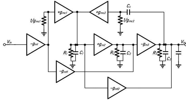
Figure 3. Topology of a three-stage ASMIHF amplifier.
