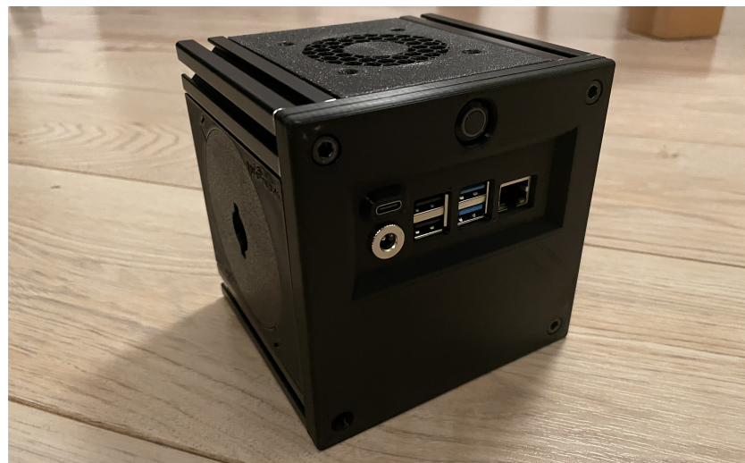
Figure 6. Photograph of the assembled Optocube housing with integrated Raspberry Pi, OptosenseCore module, OptosensePoE module, battery, ventilator, and connectors.
