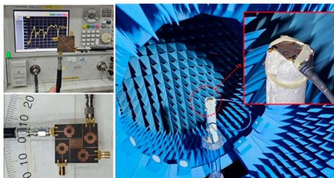
**Figure 12.** Snaps of measurement setup of the suggested MIMO Antenna.
