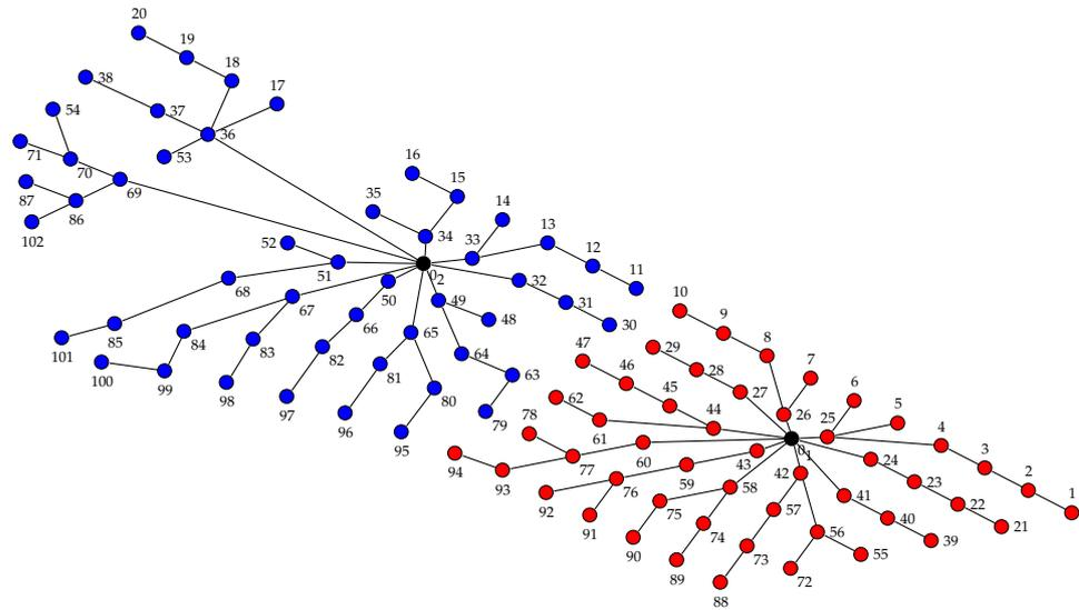
**Figure 4.** Optimal cable connection layout for WF-102-S2-W wind farm.
