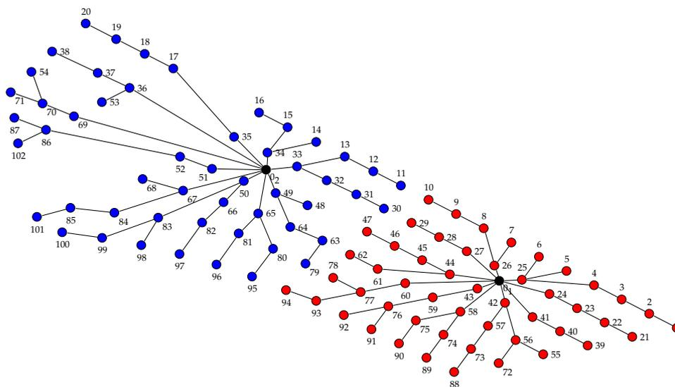
Figure 3. Optimal cable connection layout for WF-102-S2 wind farm.
