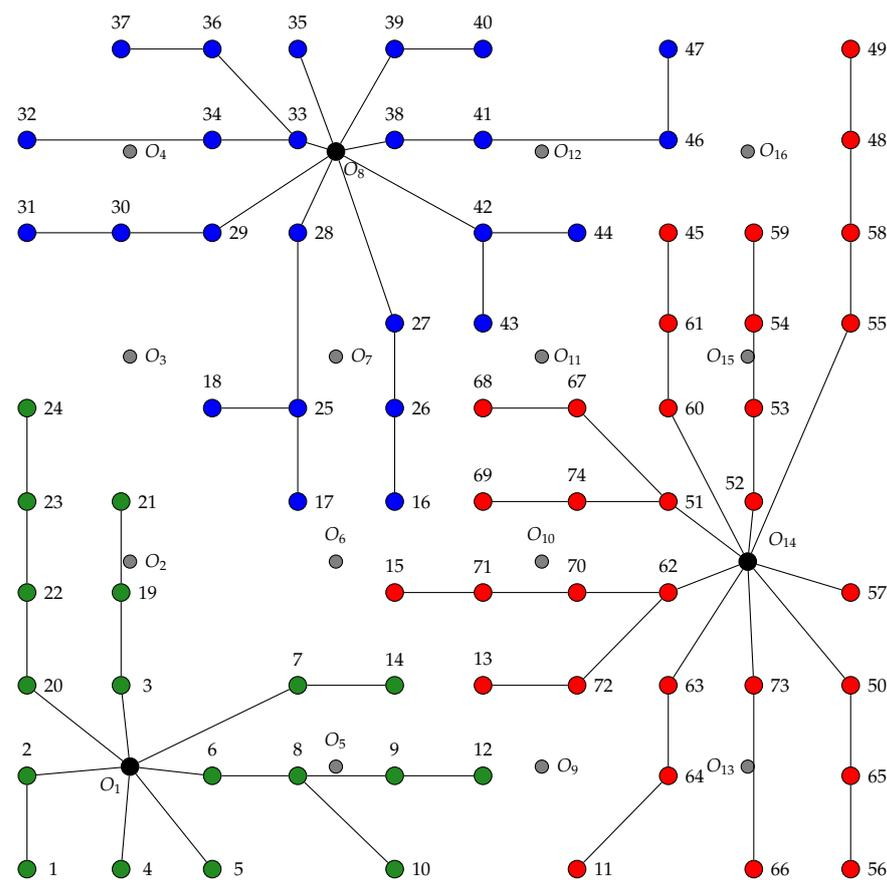
**Figure 5.** Optimal cable connection layout for the WF-74-S3 wind farm.
