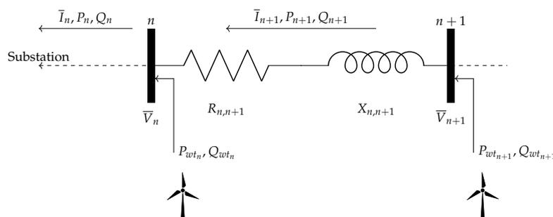
Figure 1. Line diagram of a radial distribution system.
