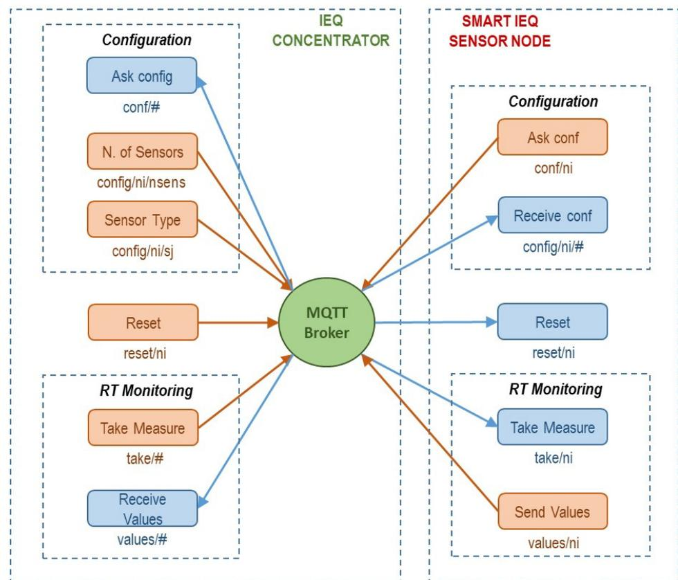
**Figure 2.** MQTT topics used for connecting IEQ concentrators with smart IEQ sensor nodes. The numbers  $i = 1, 2, 3 \dots$  represent the node identifier; the number  $j = 1, 2, 3 \dots$  represent the sensors attached to the nodes. Finally, the symbol # means being subscribed to all subtopics. Published topics are in the orange color, whereas subscribed topics are in the blue color.
