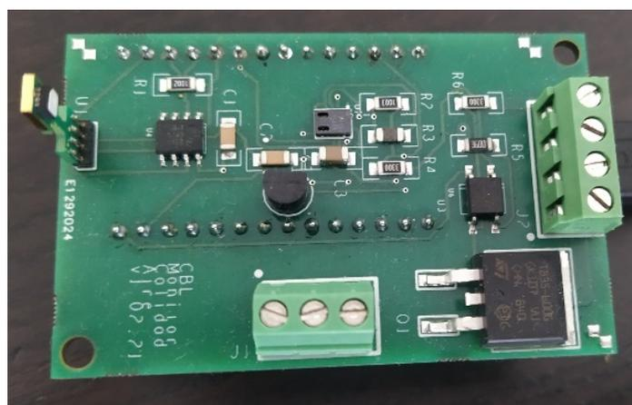
**Figure 4.** Designed PCB for the smart IEQ sensor node.
