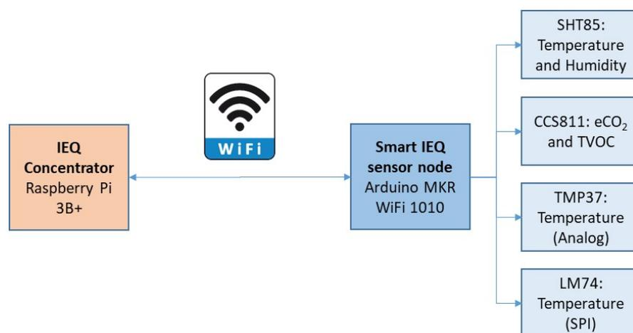
**Figure 3.** Hardware diagram for the IEQ monitoring system prototype.
