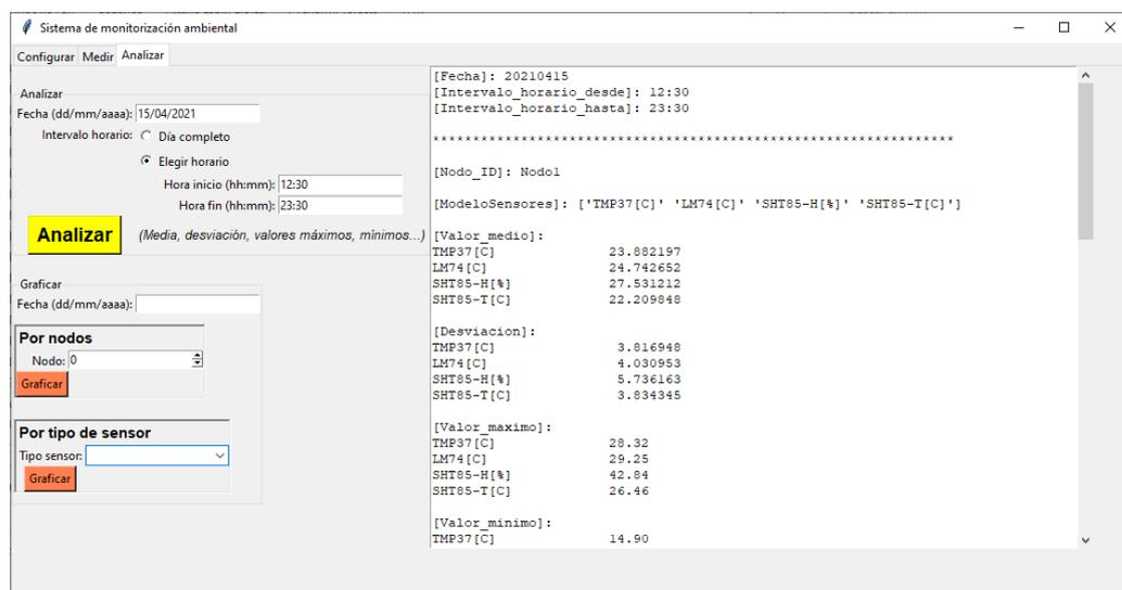
Figure 7. HMI application: Basic analysis of historical data.
