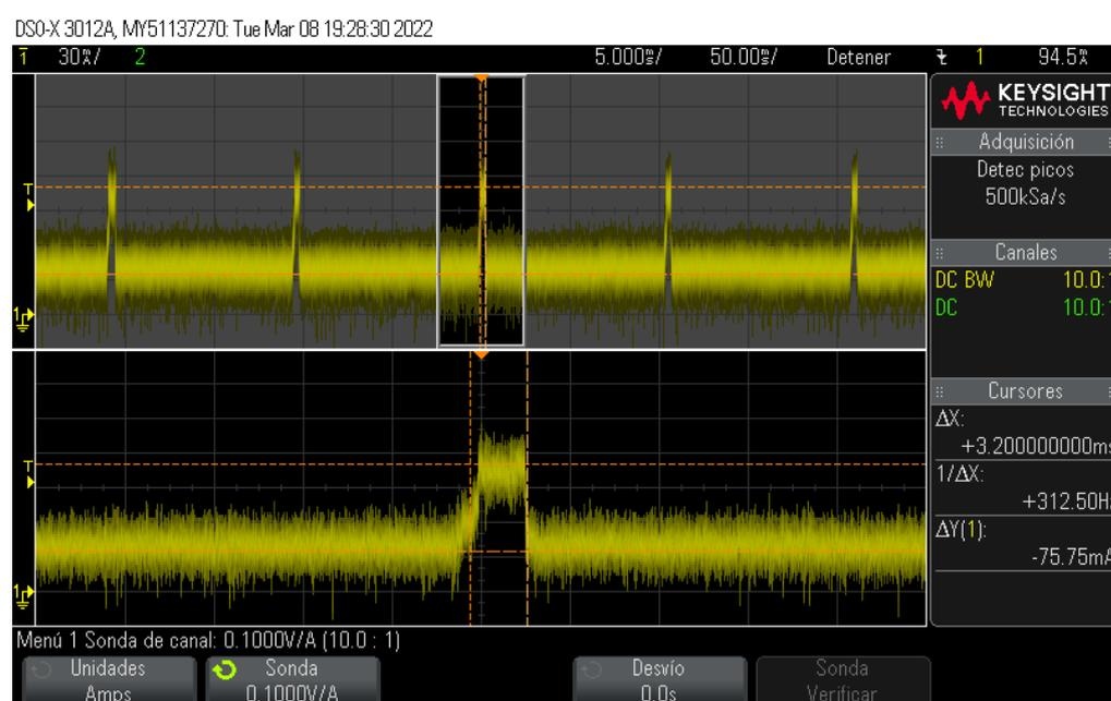
**Figure 5.** Power drawn at the smart IEQ sensor node when in operation.
