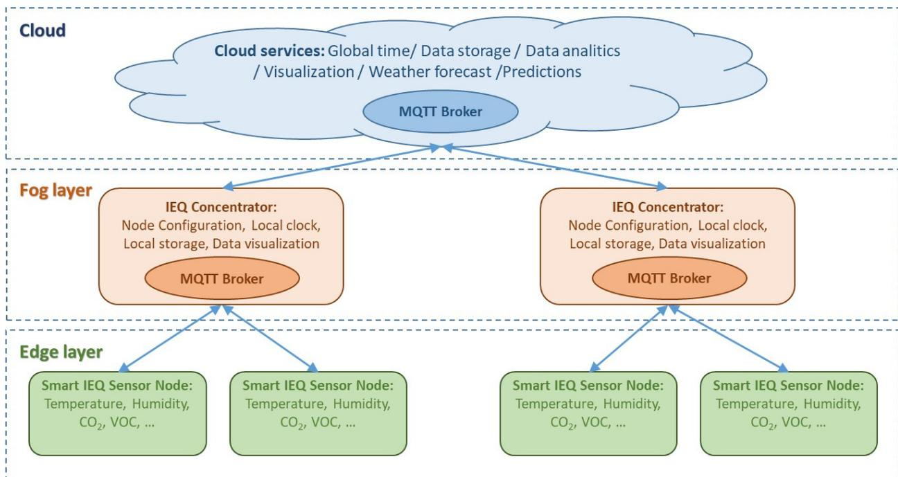
**Figure 1.** Overall architecture of the wireless acquisition system.
