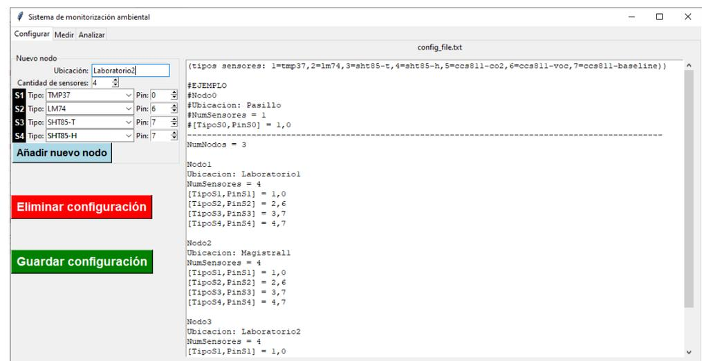
Figure 6. HMI application: Configuration of the IEQ monitoring system.
