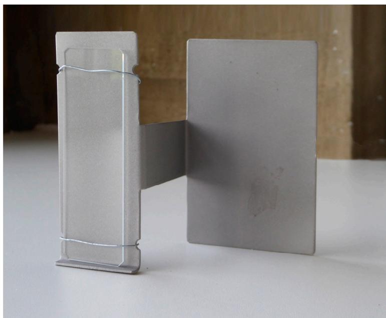
**Figure 5.** Final version of the vertical holder made of iron sheet. Note that there is a slide attached to it.
