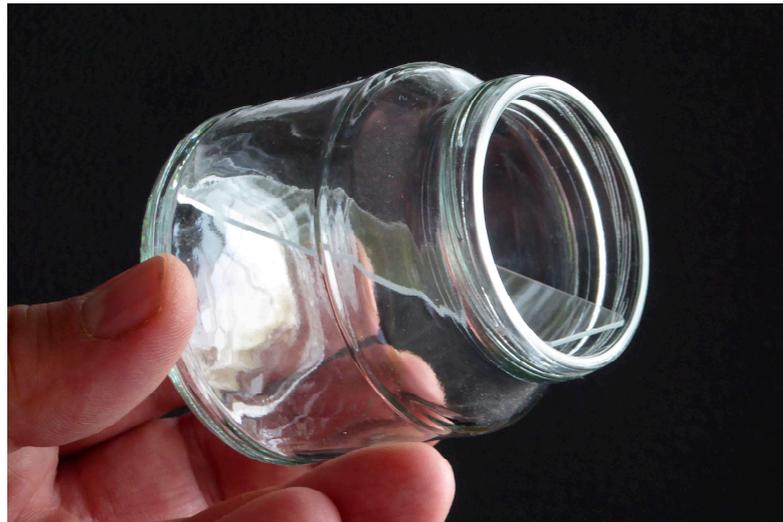
**Figure 8.** Using a glass jar to minimize contact and keep the slide horizontal.
