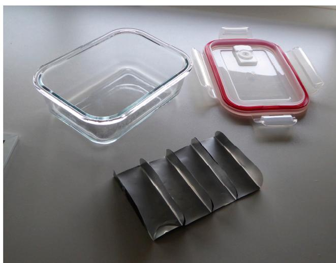
**Figure 4.** Hermetic glass storage boxes and aluminum separators used for sample collection and transportation from the cloister to the laboratory.
