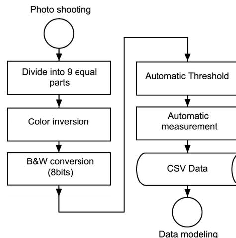
**Figure 11.** Image-processing workflow.
