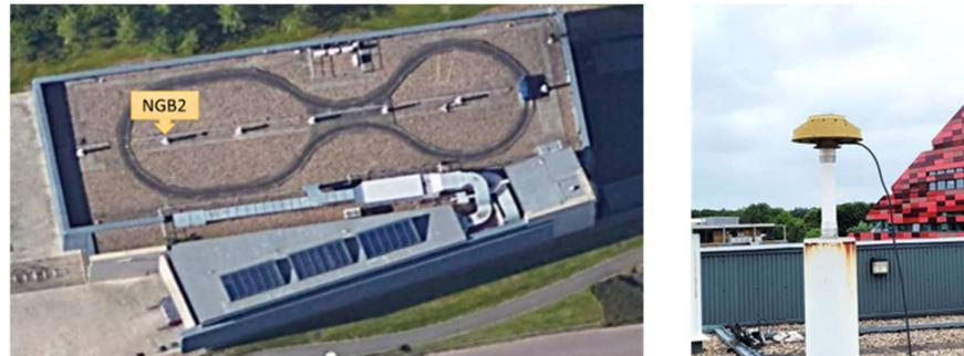
**Figure 7.** (Left) View of the roof of NGI building, with the location of control point NGB2 and (right) the GNSS antenna installed on the top of the pillar of NGB2.
