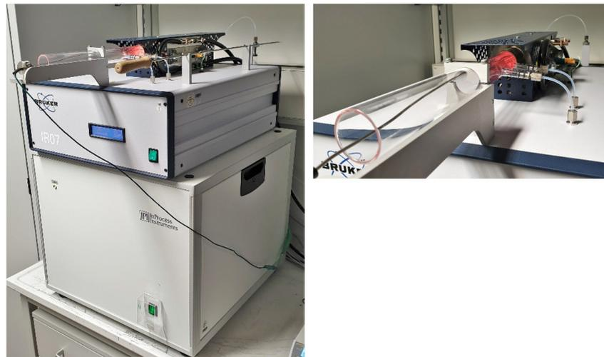
**Figure 3.** Thermal Desorption Mass Spectroscopy (TDMS).
