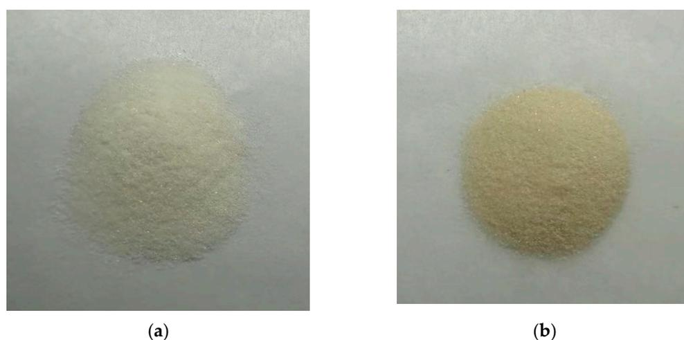
**Figure 4.** Sample photos: (a) HEC-(AA-co-AMPS) and (b) ATP-HEC-P (AA-co-AMPS).
