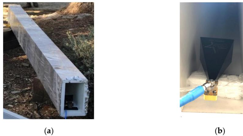
**Figure 8.** Experimental setup; (a) scaled tunnel; (b) transmitting antenna at the tunnel entrance.
