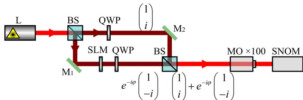
**Figure 3.** Optical setup for generating and focusing a Poincaré beam (4): L—laser with the wavelength of 532 nm; BS—nonpolarizing beam splitters; QWP—quarter-wave plate; M<sub>1</sub> and M<sub>2</sub>—rotatable mirrors; SLM—transmissive liquid-crystal spatial light modulator; MO—microobjective with a 100× zoom (NA = 0.95); and SNOM—scanning near-field optical microscope. Red arrows show the direction of light propagation.
