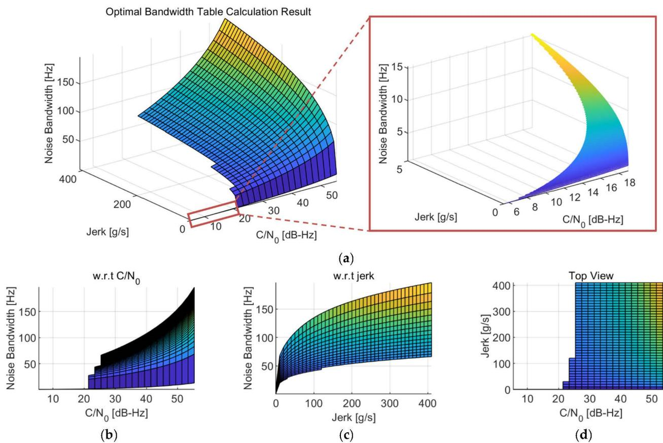
**Figure 6.** Result example of the generated optimal bandwidth table: (a) Overall shape; (b) Optimal bandwidth with respect to the  $C/N_0$ ; (c) Optimal bandwidth with respect to the jerk; (d) Top view.
