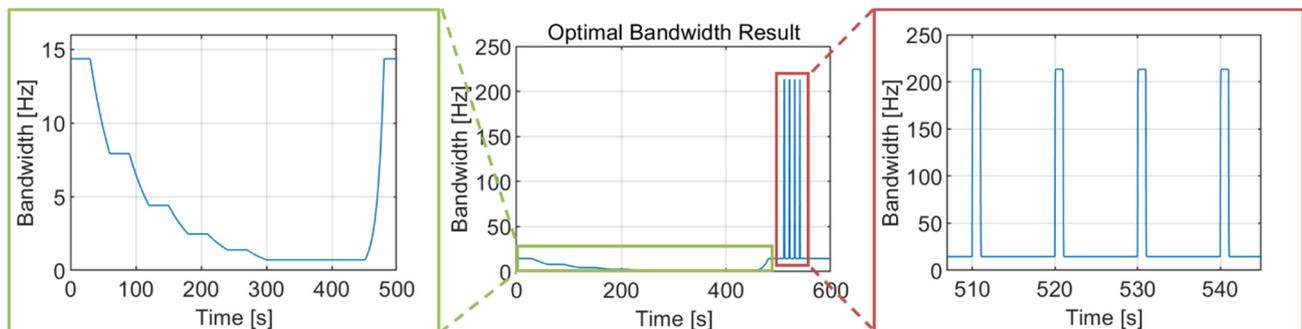
**Figure 10.** Optimal bandwidth variation during the simulation. The noise bandwidth is narrowed to 0.7 Hz as the  $C/N_0$  is lowered to 5.4 dB-Hz and widened to 213.3 Hz as the jerk dynamic stress increases to 411 g/s.
