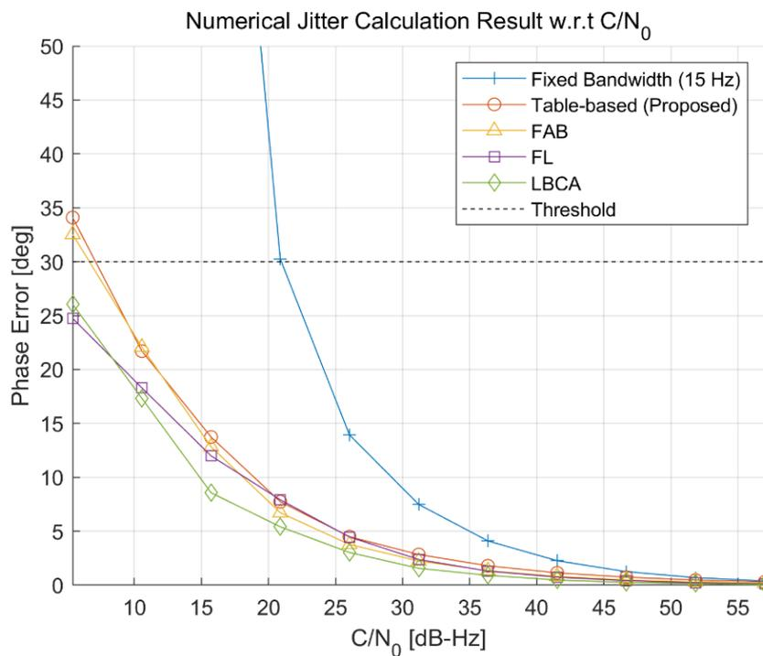
**Figure 16.** Numerical jitter calculation result with respect to the  $C/N_0$ . The proposed algorithm has a similar performance to the fast adaptive bandwidth (FAB). Fuzzy logic (FL) and loop-bandwidth control algorithm (LBCA) have slightly better performances.
