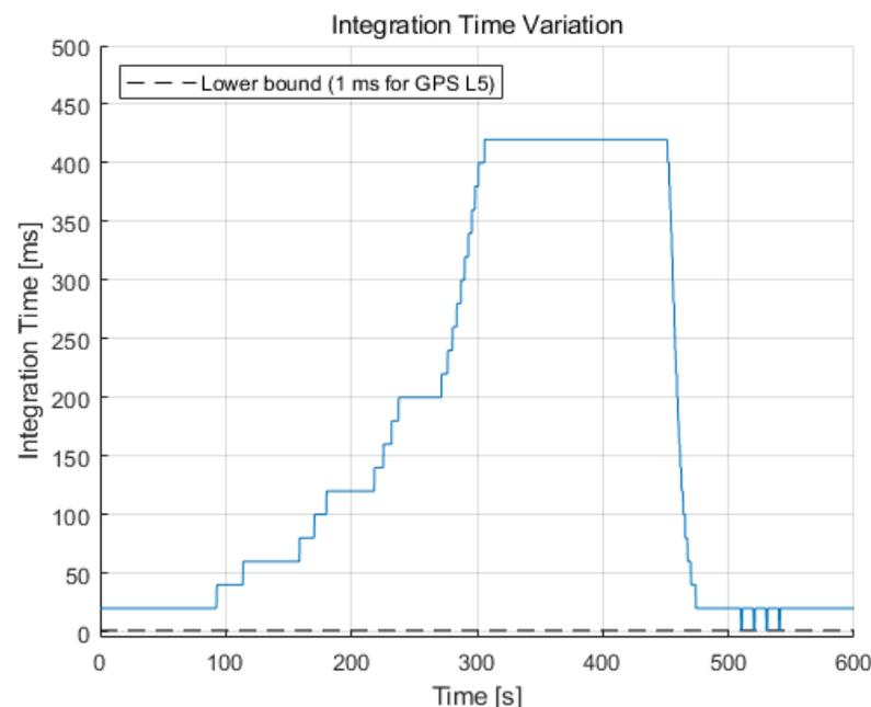
**Figure 11.** Integration time variation during the simulation varied with a step of  $\Delta T$  (20 ms for this study). It increases to 420 ms for the  $C/N_0$  of 5.4 dB-Hz and reduces to the lower bound value in the high dynamics region.
