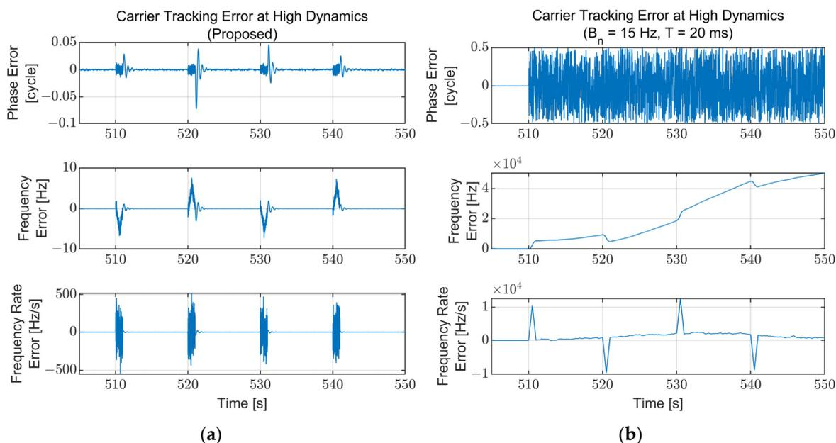
**Figure 15.** Carrier tracking error at the high dynamics region (500–550 s): (a) Proposed algorithm; (b) Fixed bandwidth ( $B_n = 15$  Hz,  $T = 20$  ms). The fixed-bandwidth loop loses lock at approximately 510 s immediately after the jerk dynamic stress occurs. The error for the proposed algorithm increases temporally while the jerk dynamic stress exists and converges to zero immediately after disappearing.
