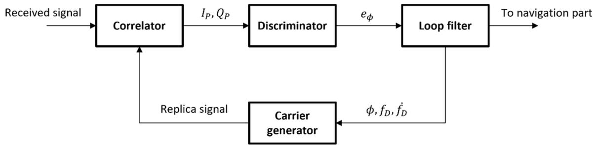
Figure 7. Simplified structure of conventional carrier tracking loop.
