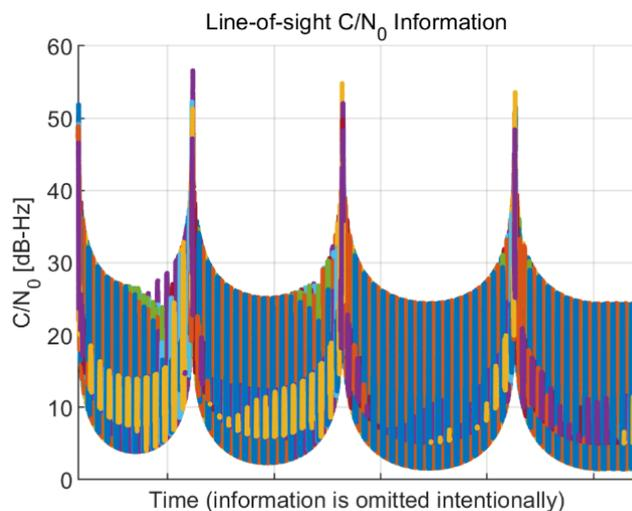
**Figure 3.** Line-of-sight (LOS) carrier-to-noise-density ratio ( $C/N_0$ ) information of the Moon exploration spacecraft during the mission trajectory. Each color in the figure indicates a different global positioning system (GPS) satellite.
