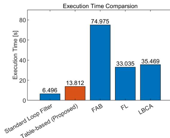
**Figure 18.** Execution time measurement results of each adaptive DPLL algorithm. The proposed algorithm has approximately 2.4–5.4 times faster execution time compared to the other adaptive DPLL algorithms.
