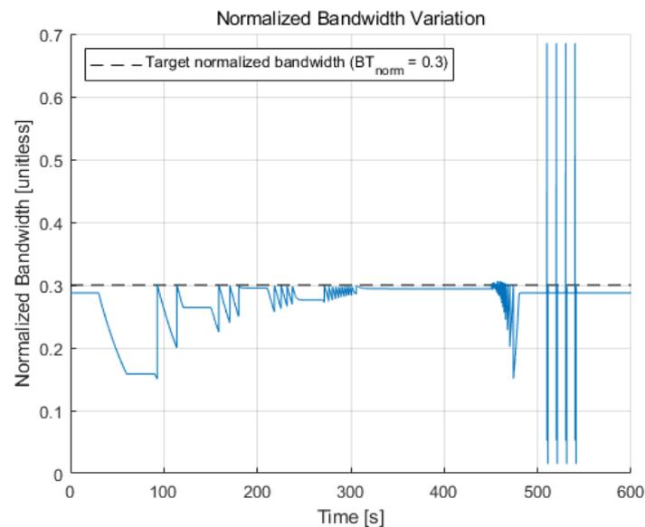
**Figure 12.** Normalized bandwidth variation during the simulation. The normalized bandwidth is maintained below the target normalized bandwidth value (i.e., 0.3) most of the time, except for the high dynamics region due to the unavoidable limitation of the integration time by the lower bound condition.
