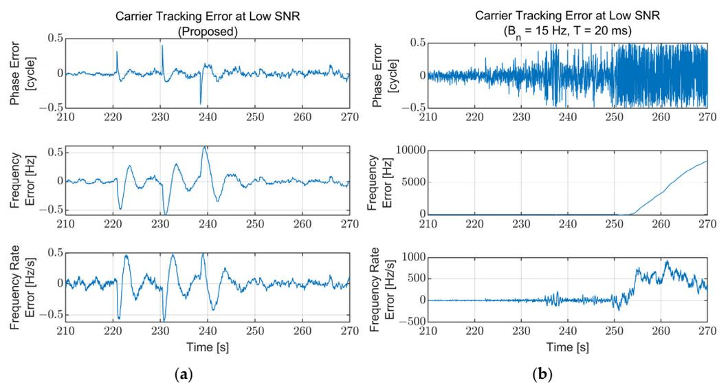
**Figure 14.** Carrier tracking error at the low SNR region (210–270 s): (a) Proposed algorithm; (b) Fixed bandwidth ( $B_n = 15$  Hz,  $T = 20$  ms). The fixed-bandwidth loop loses lock at approximately 253 s ( $C/N_0 = 17$  dB-Hz) while the proposed algorithm maintains its lock.
