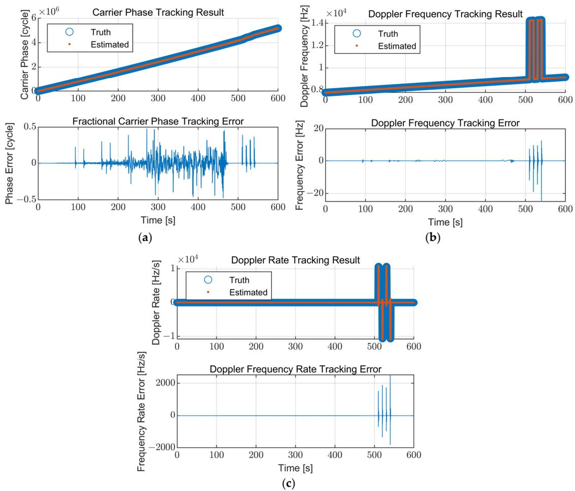
**Figure 13.** Carrier tracking results of the proposed table-based adaptive DPLL algorithm: (a) Carrier phase; (b) Doppler frequency; (c) Doppler rate. The proposed algorithm stably tracks the signal components for the simulation scenario.
