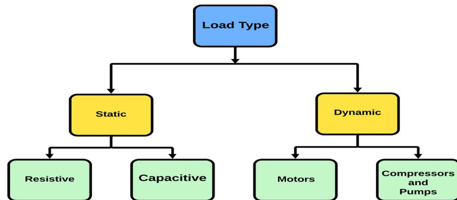
Figure 6. Microgrid load types.
