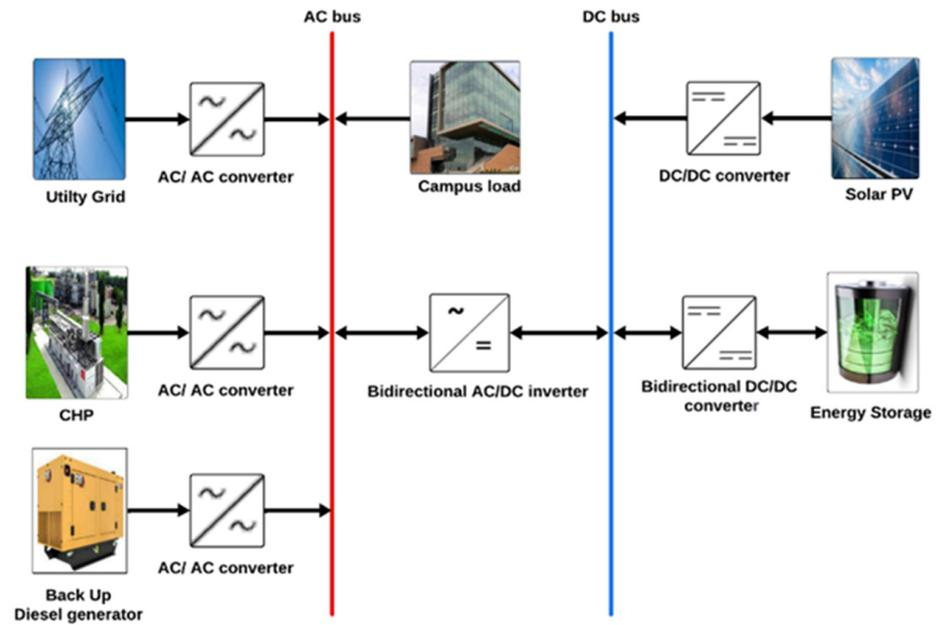
Figure 21. Microgrid connected with PV, CHP, and ESS.
