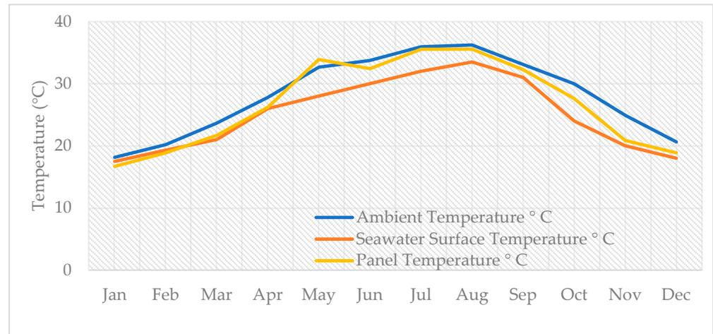
**Figure 6.** Effect of panel temperature corresponds to the seawater surface and ambient temperature.
