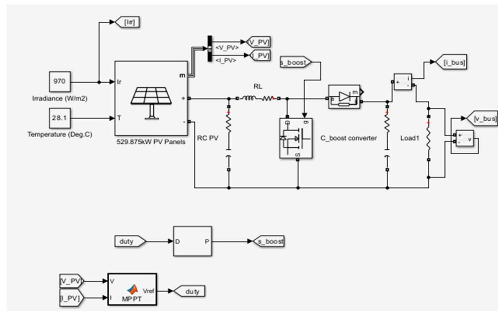
**Figure 5.** Solar PV array model using MATLAB Simulink R2022b.
