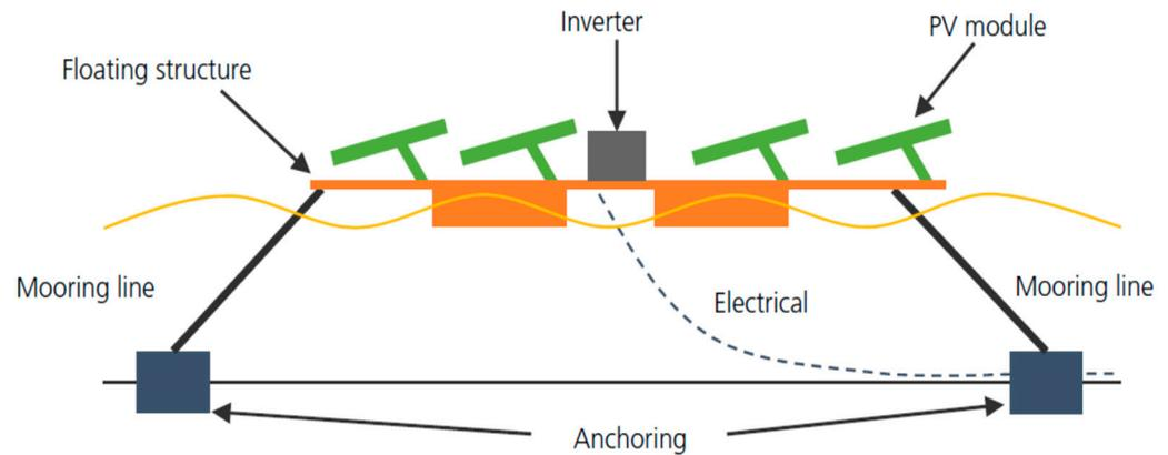
**Figure 1.** Typical floating solar PV system components.
