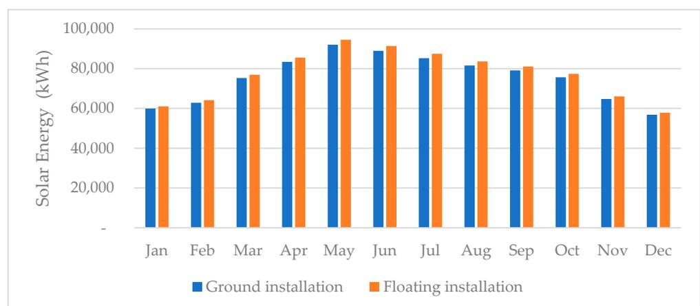
**Figure 7.** Illustration of the solar energy yield of 530 kWp floating PV system in comparison with the ground installation.
