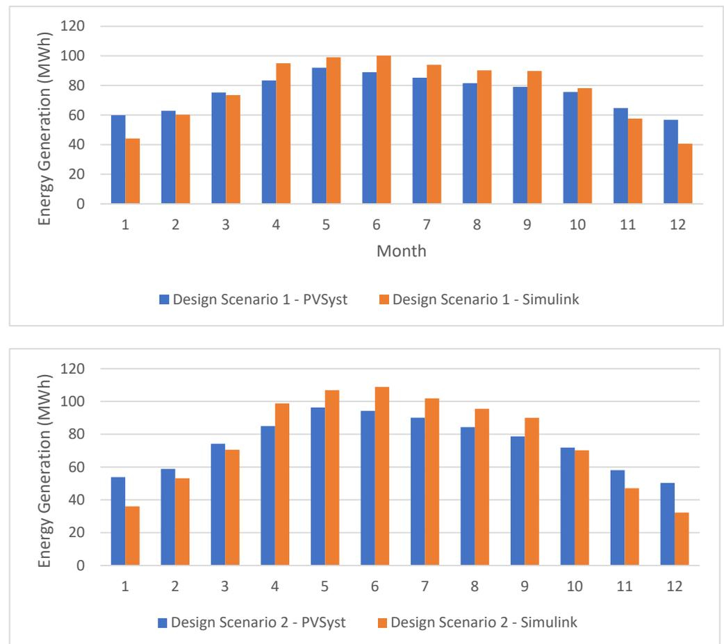
**Figure 8.** Comparison of energy generation output for design scenarios from PVsyst 7.2.21 and MATLAB Simulink R2022b.
