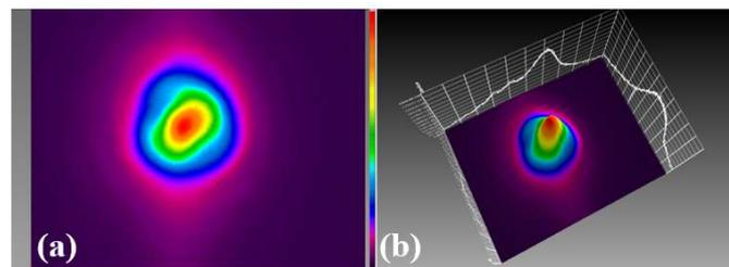
**Figure 6.** The second state of STML output pulses: (a) 2D and (b) 3D beam profiles.
