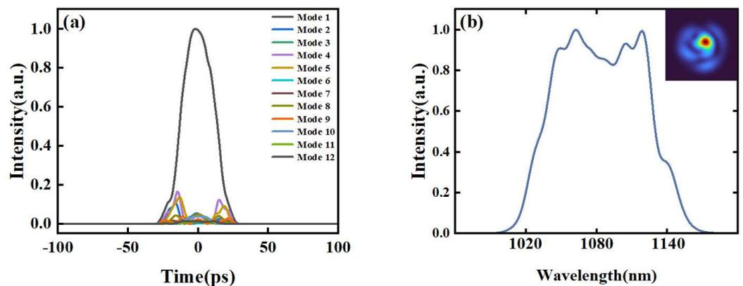
Figure 8. Intracavity spatiotemporal pulse propagation dynamics in simulations. (a) Different mode autocorrelation traces of simulated output pulses; (b) simulated optical spectrum of the output pulse, and the inset is the simulated output beam profile.
