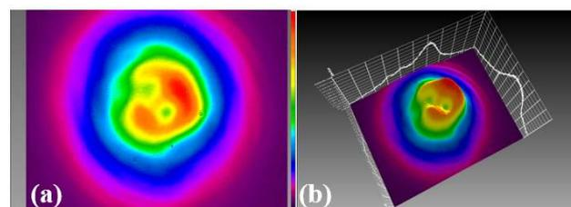
**Figure 3.** The first state of STML output pulses: (a) 2D and (b) 3D beam profiles.
