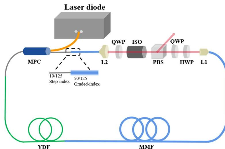
**Figure 1.** Cavity schematic of the multimode fiber laser without a spectral filter. MPC: multi-pump combiner; L1: beam collimator; L2: coupling lens; HWP: half-wave plate; QWP: quarter-wave plate; PBS: polarized beam splitter; ISO: space optical isolator; YDF: multimode gain fiber; MMF: passive graded index fiber.
