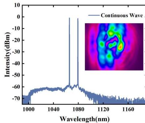
Figure 7. Continuous wave spectrum before STML, where the inset is the corresponding beam profile.
