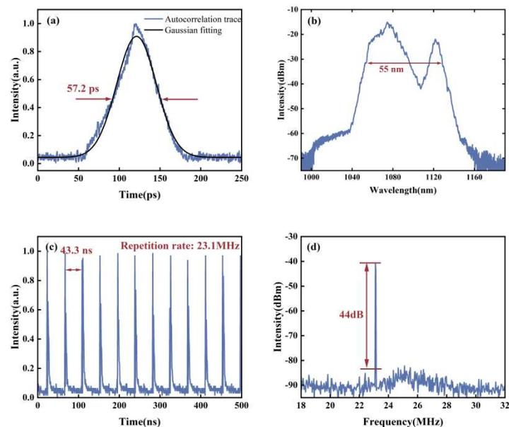
**Figure 2.** The output pulse characteristics of the first state of STML. (a) Autocorrelation trace; (b) output optical spectrum; (c) output pulse train; (d) RF spectrum.
