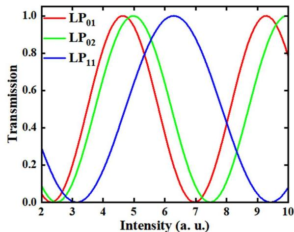
**Figure 4.** The transmittance curve distribution of the three modes ( $LP_{01}$ ,  $LP_{02}$  and  $LP_{11}$ ), obtained by normalized relative calculation based on the effective area of the  $LP_{11}$  mode.
