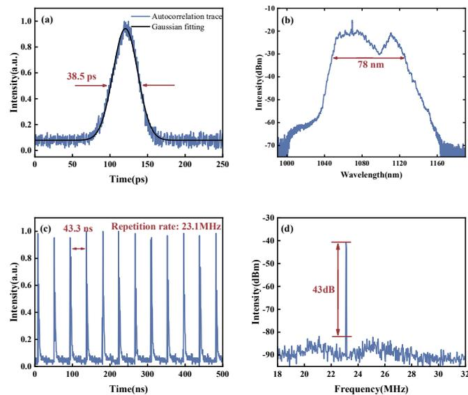
**Figure 5.** The output characteristics of the second state of STML. (a) Autocorrelation trace; (b) output optical spectrum; (c) output pulse train; (d) RF spectrum.
