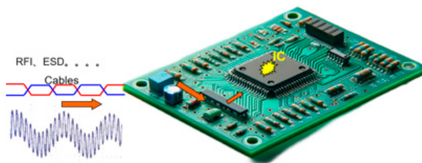
Figure 1. External interference causes sensitization of the chip on the board.
